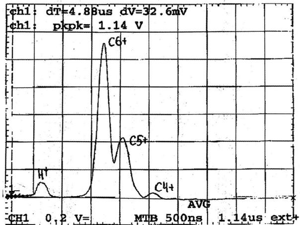
Figure 6: Ion spectra after 90 ms confinement in the electron string of the Krion-2.
