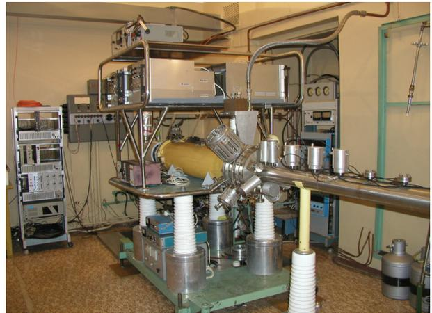
Figure 2: Electron String Ion Source Krion-2.
