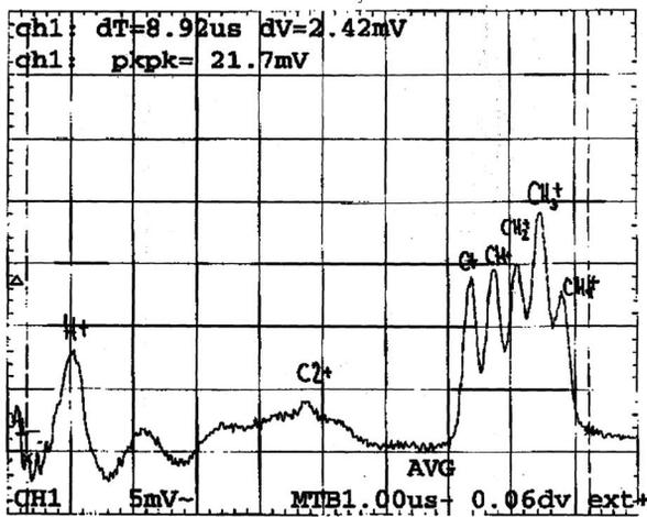
Figure 4: Ion spectra after 30  $\mu$ s methane injection into the Krion-2.
