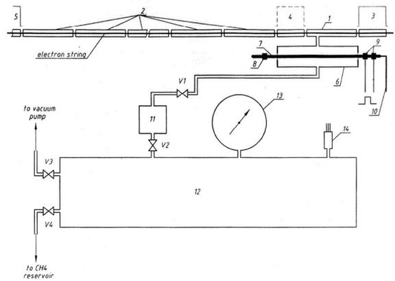
Figure 3: Scheme of Krion 2 cryogenic pulsed injection.
