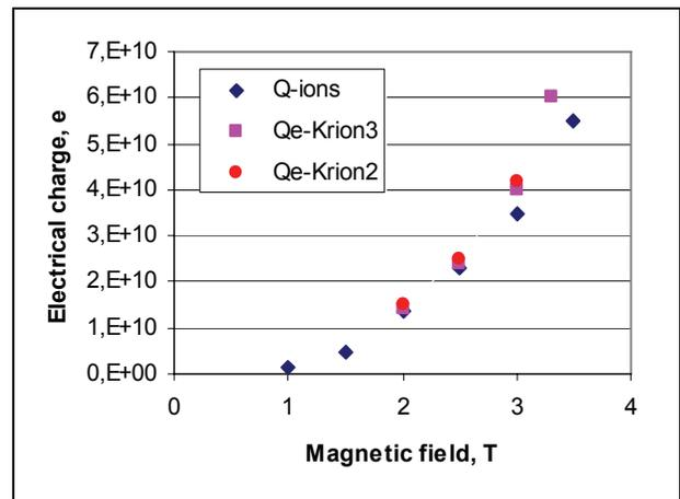
Figure 7: Dependence of the electron and ion space charge capacitances on the confined magnetic field.
