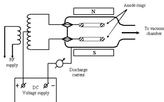
Figure 1: Double Penning vacuum cell with additional RF supply.
