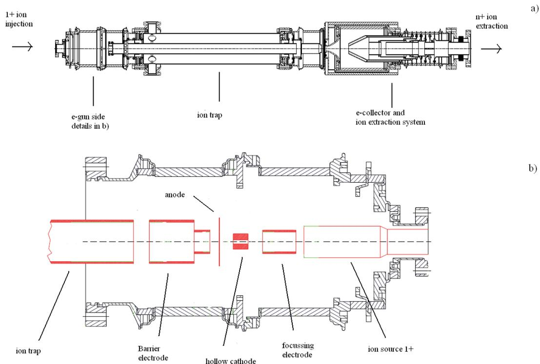
Figure 1: a) EBIS structure, longitudinal mechanical section; b) Details of the e-gun with hollow cathode. The 1+ ion source shown in the figure is a surface ion source.
