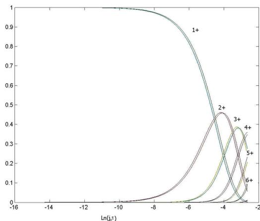
Figure 4: Ion charge state time evolution for Xe. The lower curves refer to an electron beam with hollow radius of 30% with respect to e-beam radius (upper curves).
