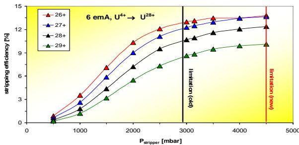
Figure 9: Yield of uranium charge states depending on nitrogen gas pressure [6].
