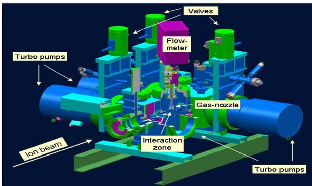
Figure 8: Improved nitrogen gas stripper chamber [4].
