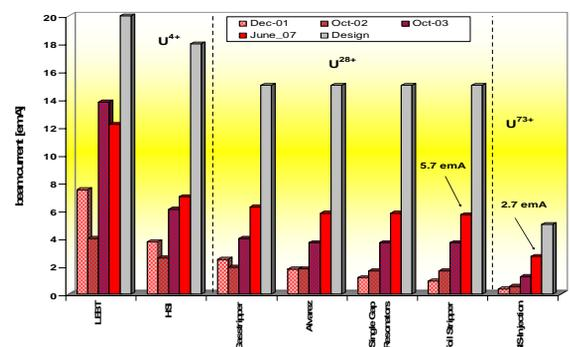
Figure 16: Improvement of the uranium beam intensities during the last years along the UNILAC [7].
