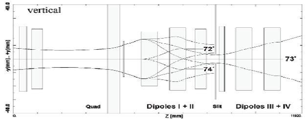
Figure 6: Beam dynamics layout of the charge state separator in the beam transfer line to SIS. Envelopes for Uranium charge states  $72+$ ,  $73+$ , and  $74+$  [6].
