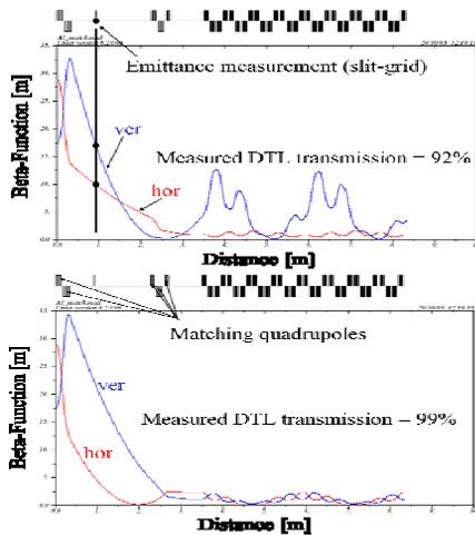
Figure 4: Horizontal and vertical beta-functions in the matching section and the first cells of the Alvarez DTL for mismatched (top) and matched (bottom) beam [2].
