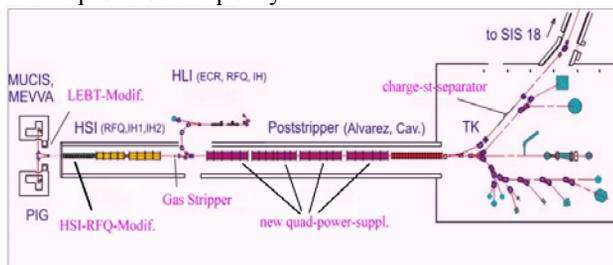
Figure 2: Schematic overview of the UNILAC, experimental area, transfer channel to SIS, and locations of upgrades.
