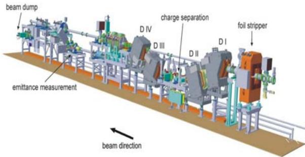
Figure 13: Charge state separator behind the foil stripper [6].
