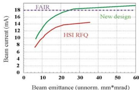
Figure 17: Simulation data of the modified HSI-RFQ (red: existing status, green: new design) [8].
