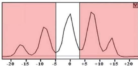
Figure 14: Measured uranium charge states 71 – 75+ [6].
