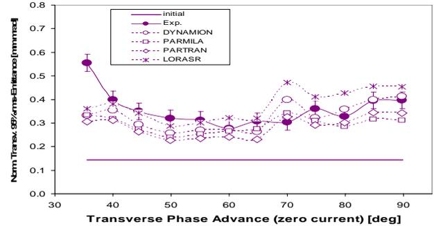
Figure 5: Transverse emittance at the exit of the Alvarez DTL calculated by different codes and measured as function of transv. phase advance.  $\epsilon_{\text{norm}} = (\epsilon_x + \epsilon_y) / 2$  [3].
