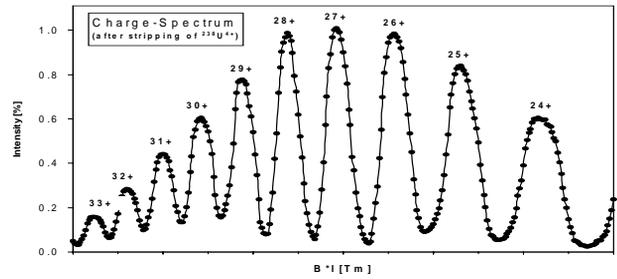
Figure 10: Uranium charge states after stripping [6].
