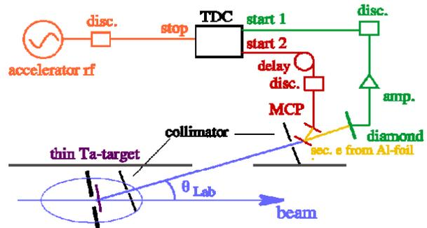
Figure 11: Scheme of the longitudinal bunch structure measurement device in front of the Alvarez DTL [5].
