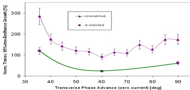
Figure 12: Measured emittance growth in the Alvarez DTL for mismatched and matched beam for different  $\sigma_0$  [3].
