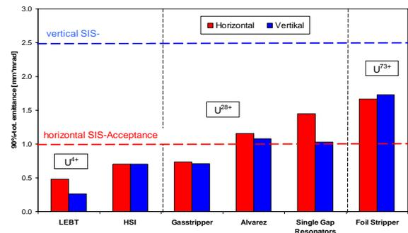
Figure 15: Normalized high current beam emittance measurements in June 2008 and SIS requirements [4].
