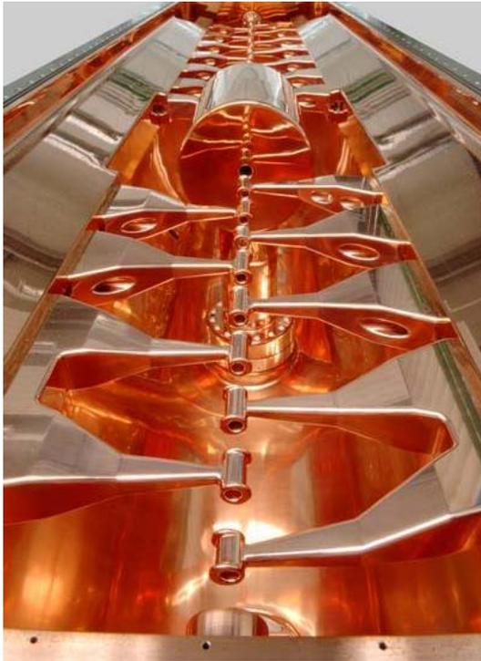
Figure 3: View into the HITRAP IH-structure from the low energy end of the resonator.
