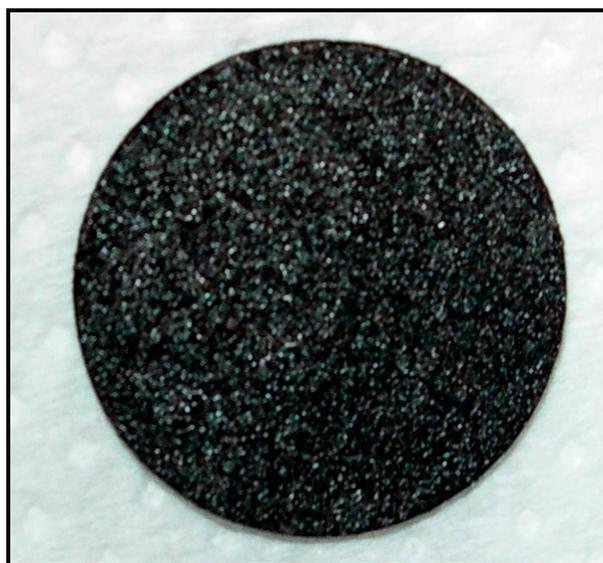
Figure 2: The first UCx pellet for the SPES project.
