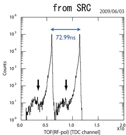
Figure 7: Longitudinal beam structure of polarized deuteron beam at the downstream of SRC. The down arrows indicate the mixture of different turn.
