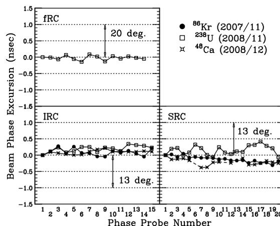
Figure 5: Isochronous condition of new cyclotrons. Data point of SRC phase probe no.6, 11, 13 in the case of  $^{48}\text{Ca}$  is not plotted because the probe was troubled by FT stray field.
