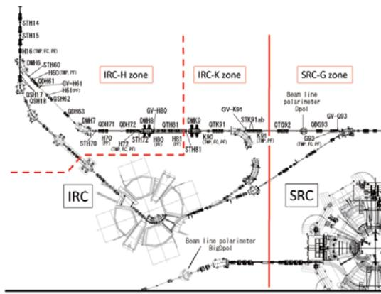
Figure 6: Schematic layout of IRC-bypass beam line used for relatively light-particle acceleration.
