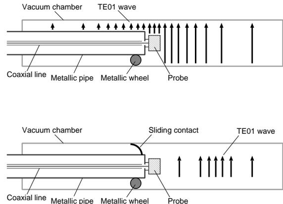
Figure 3: Effect to disturb the propagation of TE<sub>01</sub> microwave.
