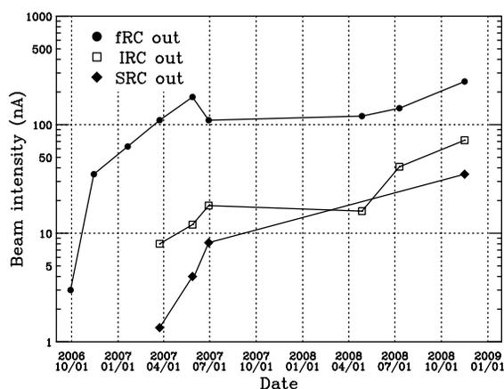
Figure 4: Evolution of maximum intensity for uranium beam during the commissioning.
