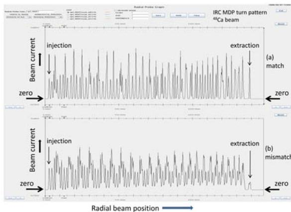
Figure 2: Radial beam pattern of  $^{48}\text{Ca}$  beam measured by MDP on IRC. FT resonator was activated. The rf phase of FT is matching in the upper panel, whereas the phase is shifted at only one degree in the lower panel.
