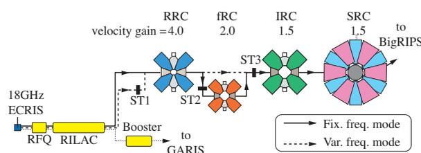
Figure 1: Conceptual layout of the accelerator chain of the RI-Beam Factory (RIBF). A linac injector (RILAC) is followed by the booster cyclotrons: RRC (RIKEN Ring Cyclotron, K540 MeV), fRC (fixed-frequency Ring Cyclotron, K570 MeV), IRC (Intermediate-stage Ring Cyclotron, K980 MeV), and SRC (Superconducting Ring Cyclotron, K2600 MeV). The charge strippers are indicated by ST1 - ST3.
