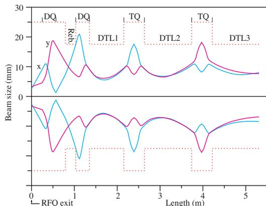
Figure 9: Calculated beam envelopes in the DTL. The emittance ellipses were assumed to be  $0.6 \pi$  mm-mrad (normalized) in both of the transverse planes.
