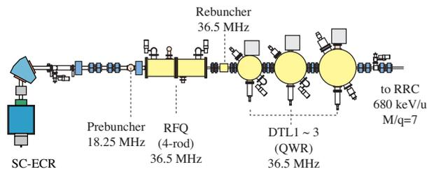
Figure 6: Schematic drawing of the new injector.
