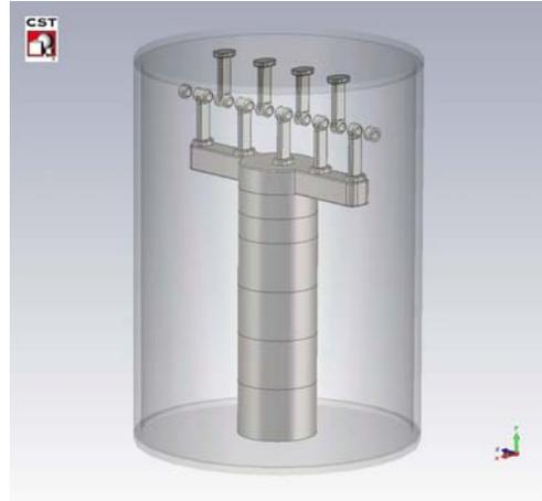
Figure 8: Schematic drawing of the DTL resonator.
