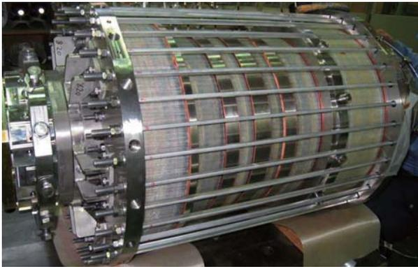
Figure 2: Superconducting coil of the ECR ion source.
