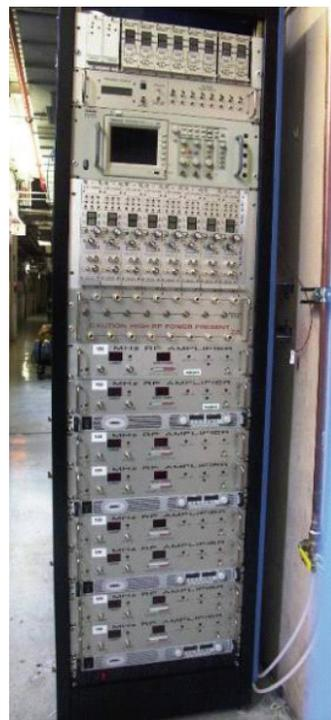
Figure 3: The main RF rack containing 109 MHz amplifiers and control modules.
