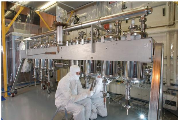
Figure 1: The cavity string assembly in the clean area is complete, including complete, sealed cavity vacuum system.
