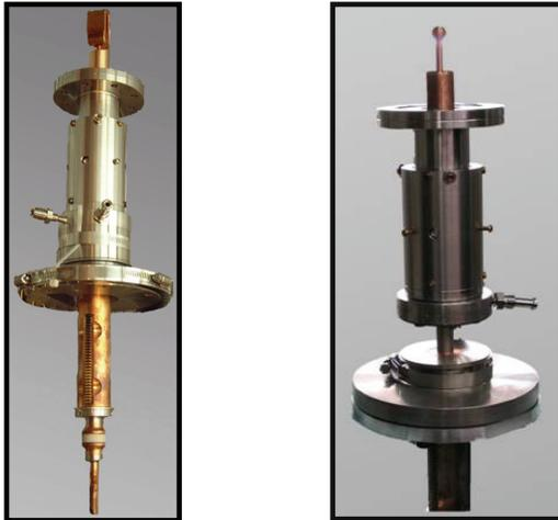
Figure 5: Inductive coupler on the left and a capacitive coupler on the right.
