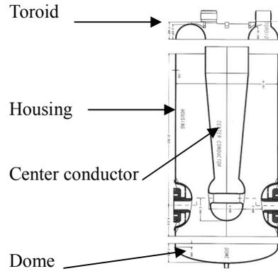
Figure 1: Four main cavity sections.
