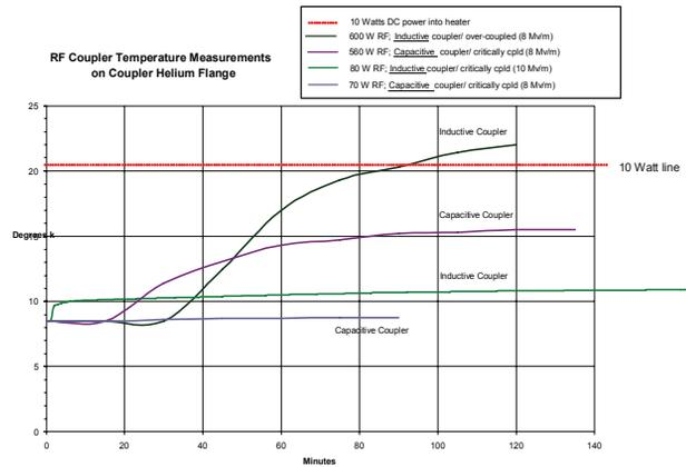
Figure 7: RF Coupler heating at the 4.5K flange.
