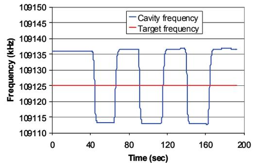
Figure 4: Typical slow tuner range measured at 4.5K.
