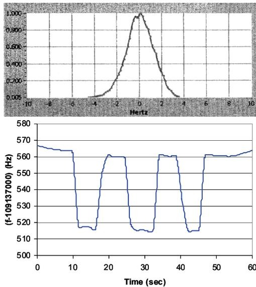
Figure 8: Top, measured frequency deviation from microphonics. Bottom, measured fast tuner window.
