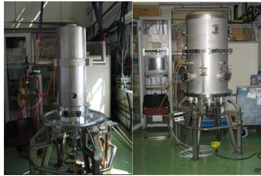
Figure 8: On the left the dummy cavity during mounting for the first sputtering. On the right the sputtering chamber closed.
