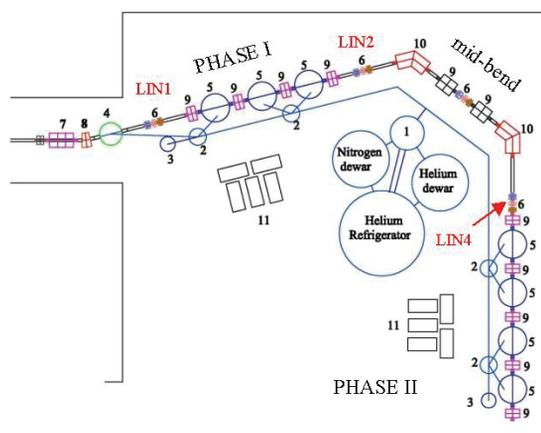
Figure 1: A schematic layout of the LINAC.
