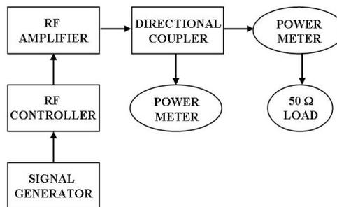
Figure 3: Power setting procedure for the QWR.
