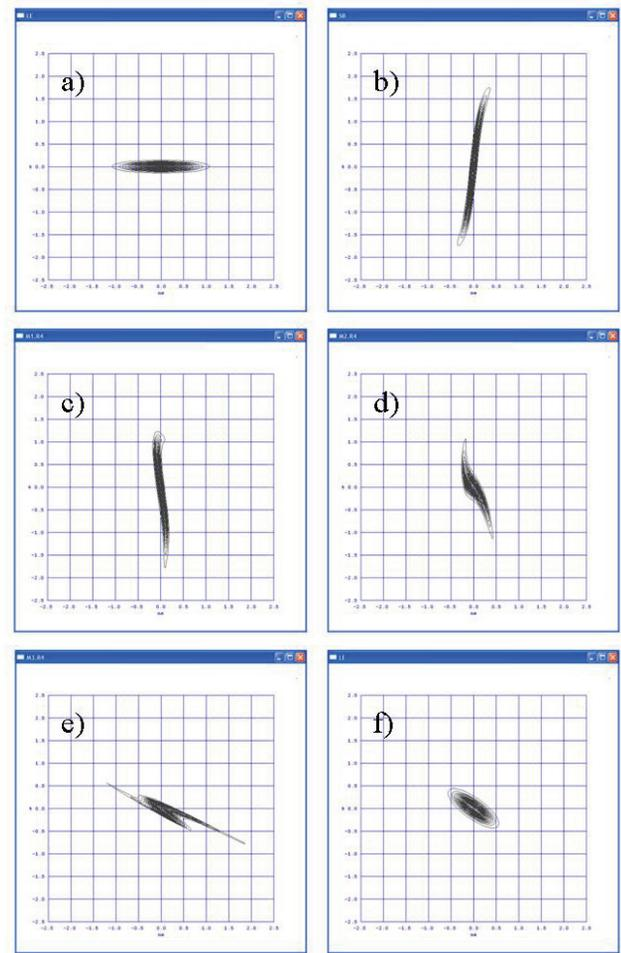
Figure 4: Longitudinal phase space (see text for details): a) at LINAC injection, b) after Superbuncher, at the entry of M1, c) after M1, at the entry of M2, d) after M2, at the entry of M3, e) after mid-bend, at the Phase II entry, f) equivalent distribution for the Phase II corresponding to (e).
