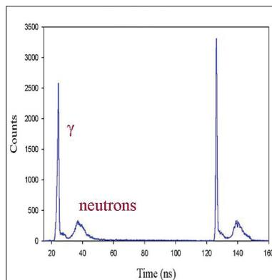
Figure 6: Time spectrum with BaF<sub>2</sub> detector at target position ( $\sigma_{beam} \sim 250$  ps).
