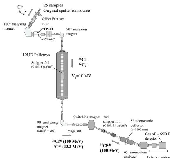
Figure 3: Schematic diagram of the Tsukuba AMS system. Labels indicate the main components along the AMS beam line and the experimental setup for AMS measurements of  $^{36}\text{Cl}$ .
