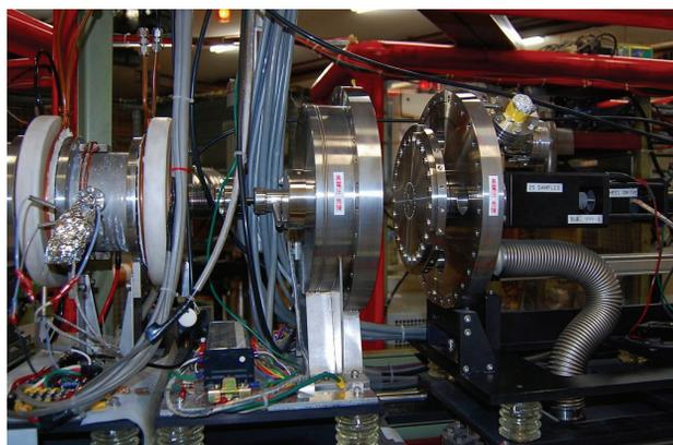
Figure 4: A 25-sample holder of an original Cs sputtering ion source for AMS.
