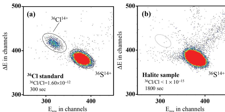
Figure 7: (a)  $^{36}\text{Cl}$  spectrum of a standard sample for  $^{36}\text{Cl}/\text{Cl} = 1.60 \times 10^{-12}$ . (b)  $^{36}\text{Cl}$  spectrum of a halite sample for the system background check. Total 3 counts of  $^{36}\text{Cl}$  are detected for 30-minute measurement. The background level is lower than  $^{36}\text{Cl}/\text{Cl} = 1 \times 10^{-15}$ .
