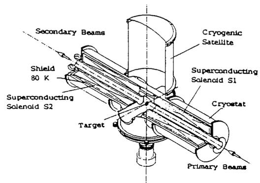
Figure 2: Schematic view of the cryostat of SISSI.
