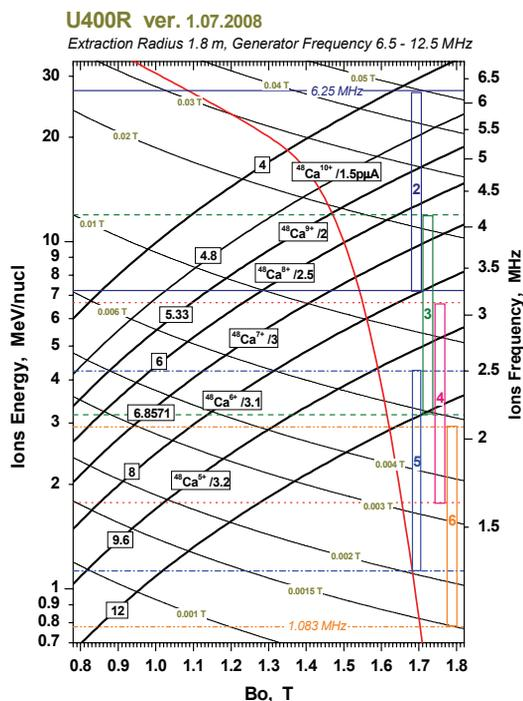
Figure 3: Operating chart of the U400R cyclotron.
