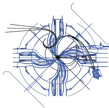
Figure 5: Scheme of beam extraction from U400M.
