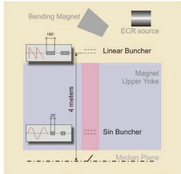
Figure 2: Scheme of the beam bunching system.
