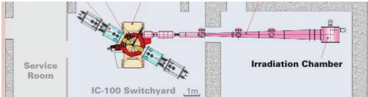
Figure 6: Plan of a specialized complex for applied research based on the IC100 cyclic implanter.
