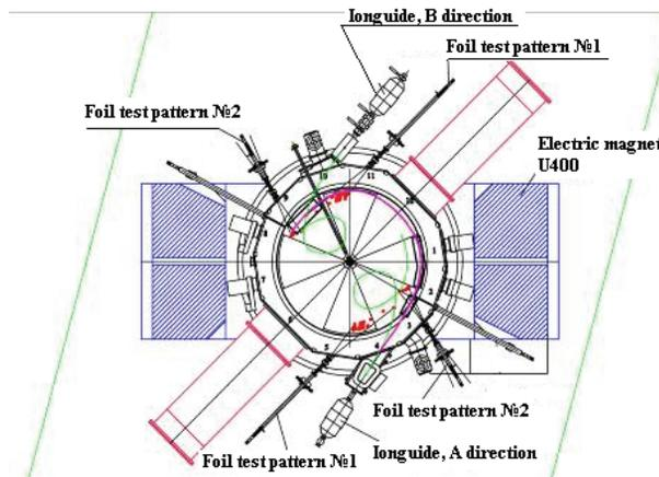
Figure 4. Scheme of the beam extraction in two selected directions.
