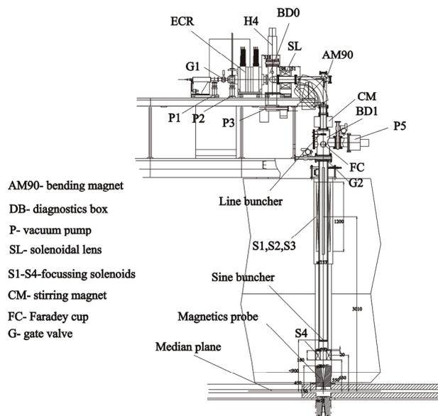
Figure 7: Scheme of U400R axial injection system.
