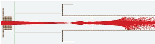
Figure 5: 1+ trajectories without decelerating tube.
