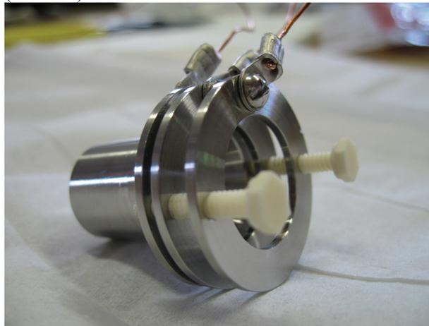
Figure 2: Small Faraday cup which was inserted into the transfer tube. The cup has an isolated ground ring, suppressor ring at -300 V, and isolated collector. The cup acceptance ( $\Phi$  19 mm) matches that of the transfer tube.
