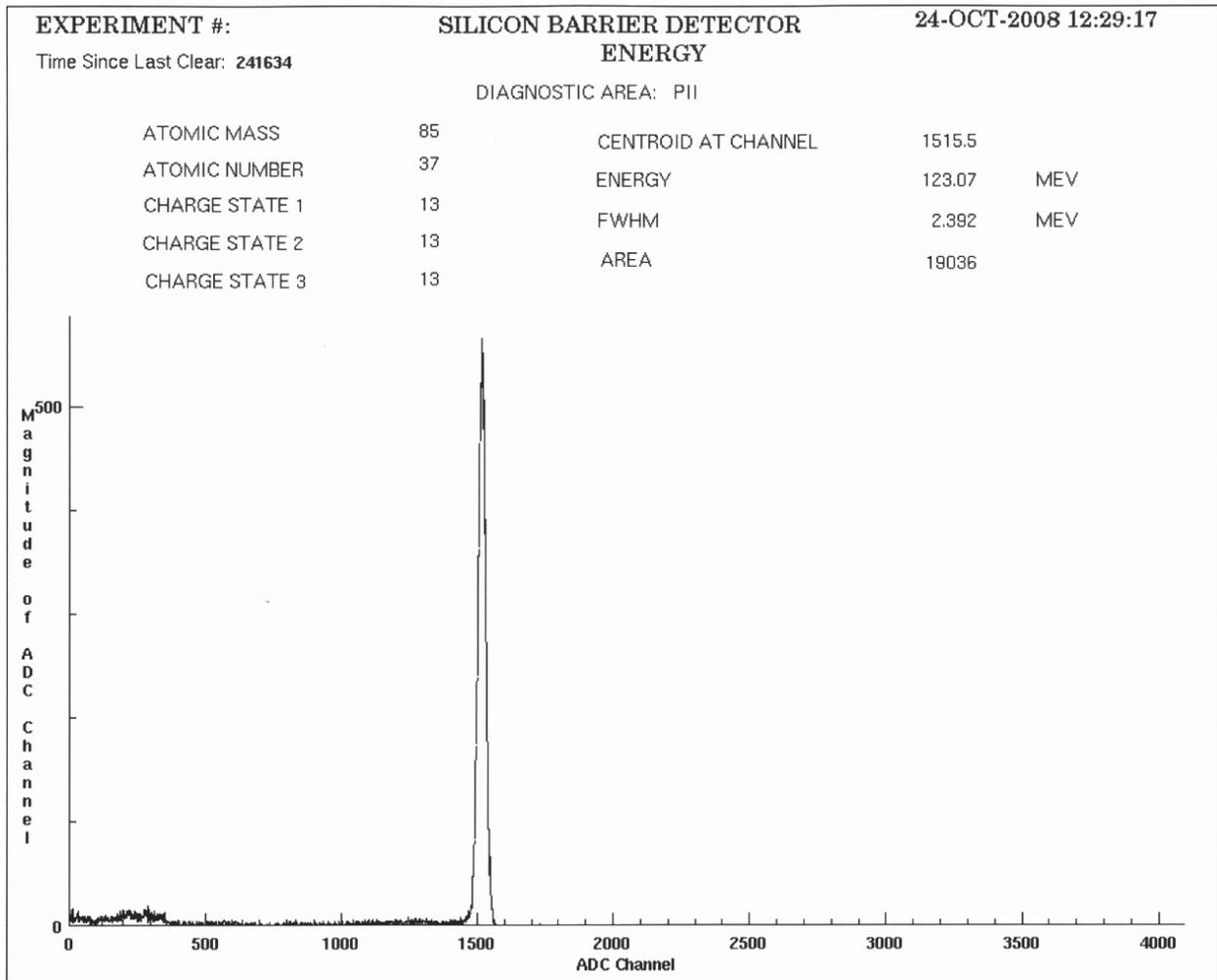
Figure 4: Energy Spectrum of charge bred  $^{85}\text{Rb}^{13+}$  after acceleration through the Positive Ion Injector Linac of ATLAS showing an exit energy of 123.07 MeV(1.45 MeV/u).
