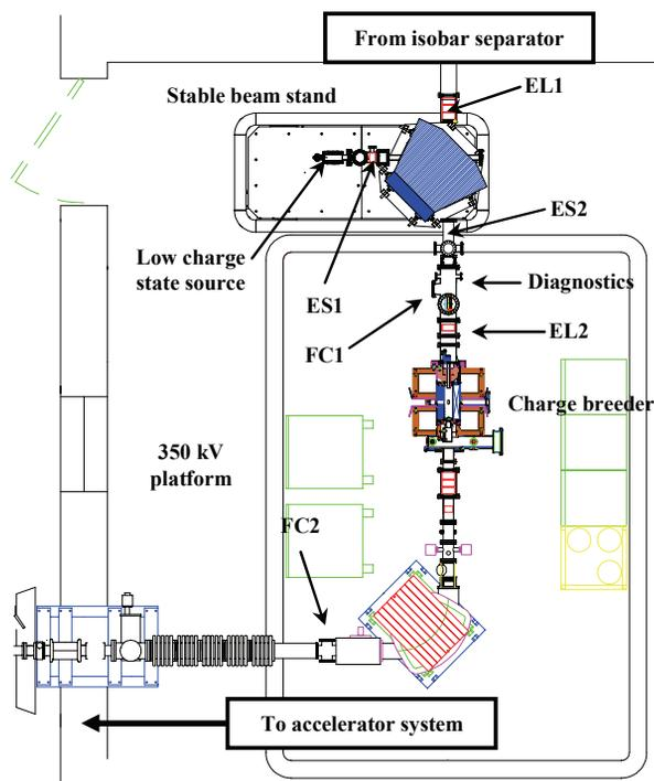
Figure 1: Floor plan of the charge breeder system showing the stable beam stand and surface ionization source, the electrostatic steerers (ES1 and ES2), the einzel lenses (EL1 and EL2), the Faraday cups (FC1 and FC2), the diagnostics location (emittance), and the ECR charge breeder.
