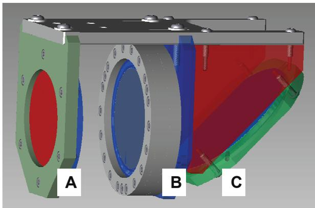
Figure 5: Schematic of the pepper pot emittance device constructed for the 1+ and charge bred beams. Item A is the mask, B is the CsI crystal and C is a mirror.
