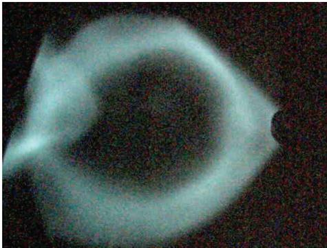
Figure 9: A hollow  $\text{Ar}^{8+}$  ion beam after dipole.
