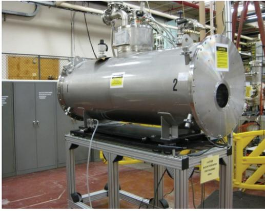
Figure 11: The 5 T, 2 m long EBIS solenoid at BNL.
