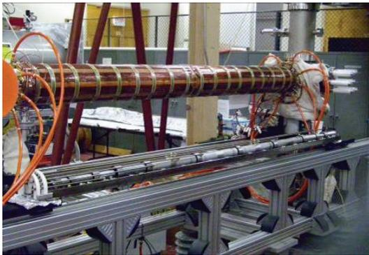
Figure 12: EBIS drift tube structure (below) and central vacuum chamber (above) where it will be inserted.
