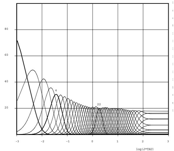
Figure 3: Charge breeding of lead at 5025 eV electron energy including charge exchange at a pressure of  $10^{-8}$  mbar.
