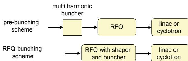
Figure 5: Schemes of micro bunching of the ion beams extracted from EBIS/T and ECRIS devices using an external buncher-RFQ combination or an RFQ with shaper and buncher section.
