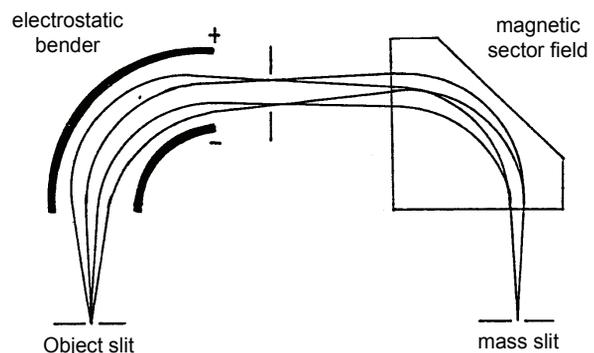
Figure 4: Principle of an achromatic Q/A-separator or a separated function velocity filter.
