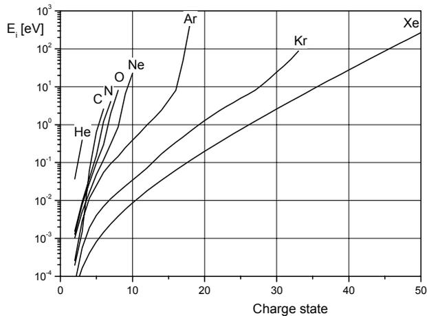
Figure 1: Ion energies by Coulomb collisions with 3 keV electrons during stepwise ionization.
