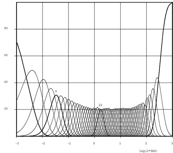
Figure 2: Charge breeding of lead at 5025 eV electron energy, without radiative recombination and without charge exchange.
