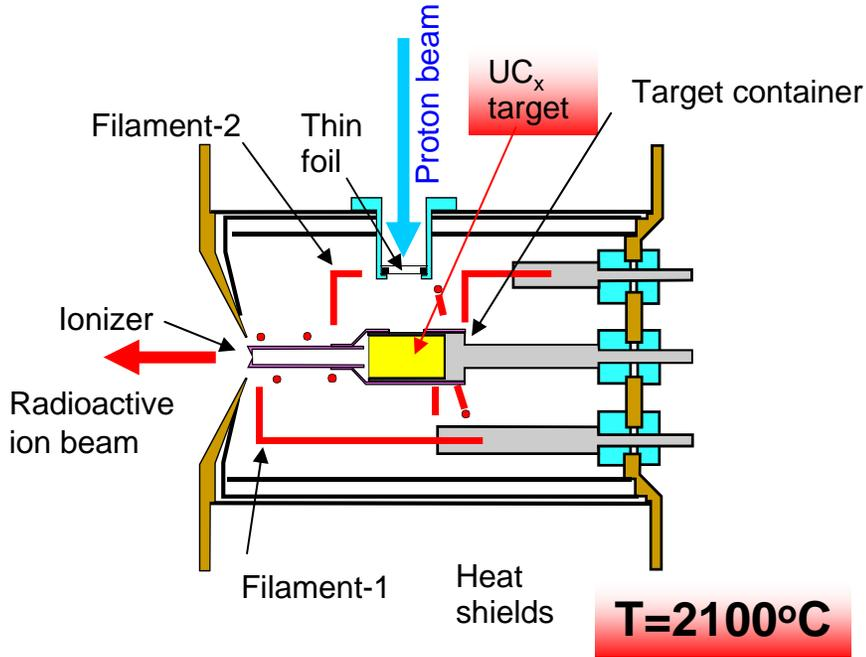
Uranium Target-Surface Ionization IS
