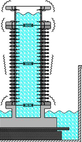
Remove micro-particles on the inside tube wall
