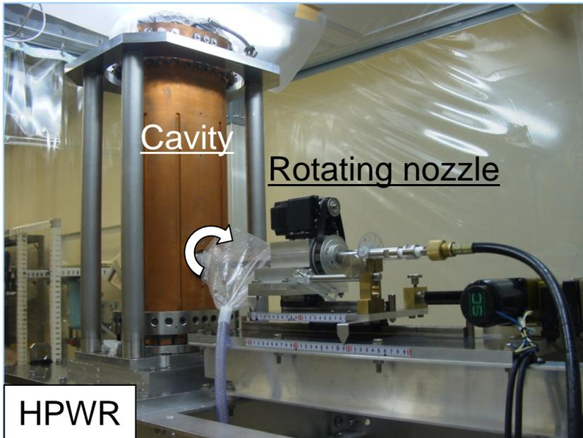
Water flow: 6 l/m, Pressure: 6~8 MPa
