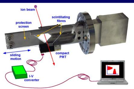
**Beam profile monitor** based on a pair of scintillating fibres scanning the beam
