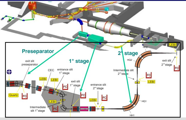
The mass separator system consists of a pre-separator and 2 main stages, the pre-separator and the first stage being assembled on two 250 kV platforms
