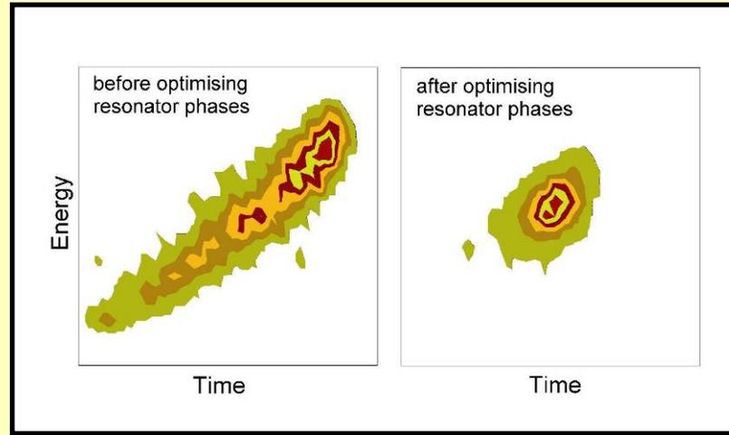
*Longitudinal phase space after mid-bend (E-T measurement)*
