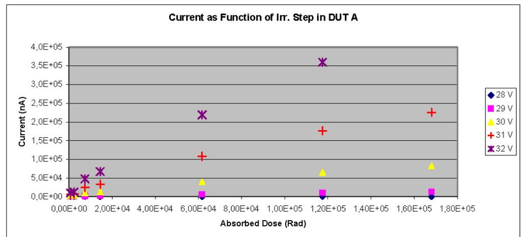
Figure 10 DUT A current as a function of irradiation step at various Bias values around break-down; notice that at 32 V the current was too high for the source meter after step 6.
