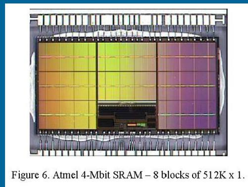
Figure 6. Atmel 4-Mbit SRAM – 8 blocks of 512K x 1.
