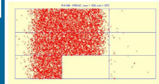
Figure 8. Physical location of SEUs – revealing a faulty beam.
