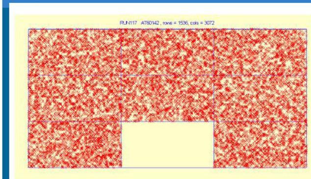
Figure 7. Physical location of SEUs - confirming uniform beam.
