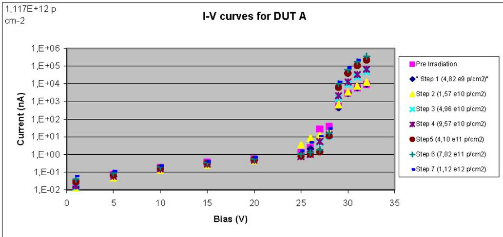
Figure 7 I\_V curves for device A prior to irradiation and after each step.
