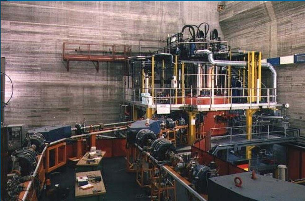
The **LNS Cyclotron** has 15 to 48 MHz RF system;
