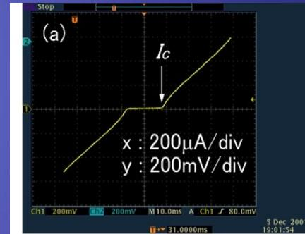
Characteristics of SQUID. The response of the sensitive SQUID loop is periodic with respect to a magnetic flux quantum,  $\Phi_0 = h/2e = 2.068 \times 10^{-15}$  weber.
