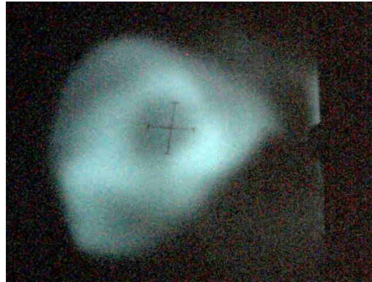
Location of focal point depends on the charge state: higher charge state can “explode” lower charge state if intensity high enough
