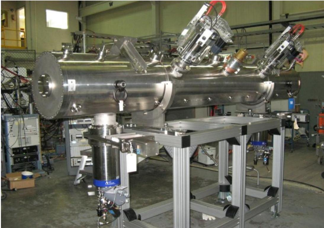
*The RFQ has successfully accelerated He, Cu, & Ne from the Test EBIS at BNL.*
