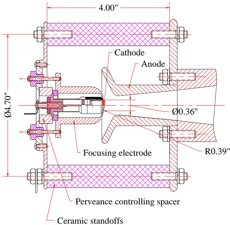
The present cathode is actually capable of operating at 20 A ( $J=30A/cm^2$ ) with lifetime of 3000-5000 hours. For possible future increase of the ion beam intensity, we have built the electron gun electrodes and collector with the capability of operating at 20A.
