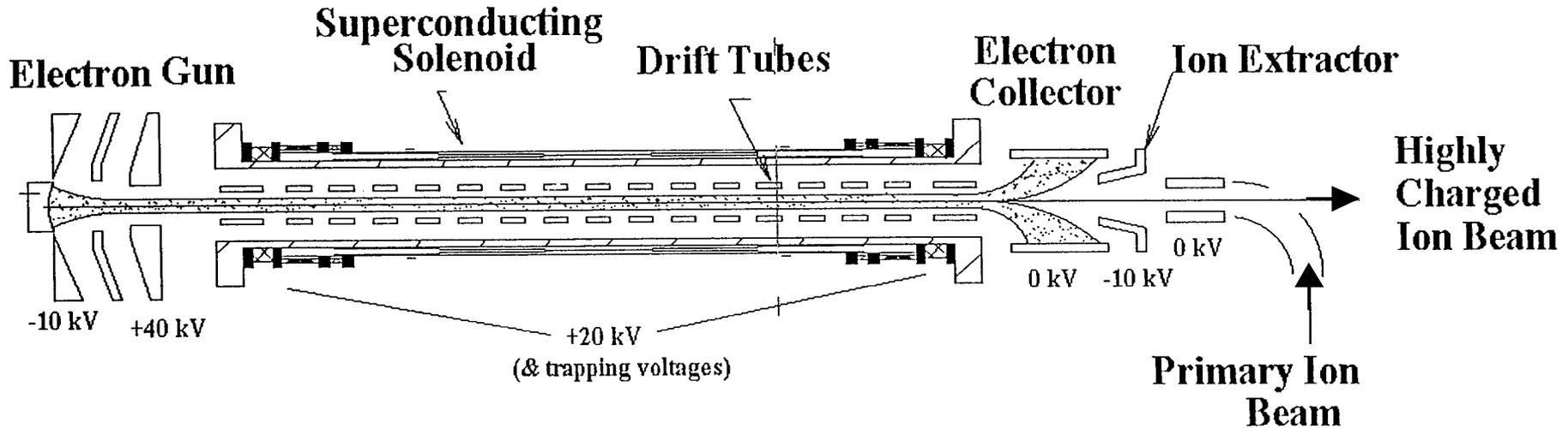
**Radial trapping of ions by the space charge of the electron beam.**
