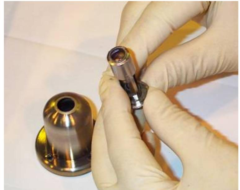
9.2 mm diameter convex cathodes (LaB<sub>6</sub> shown)
