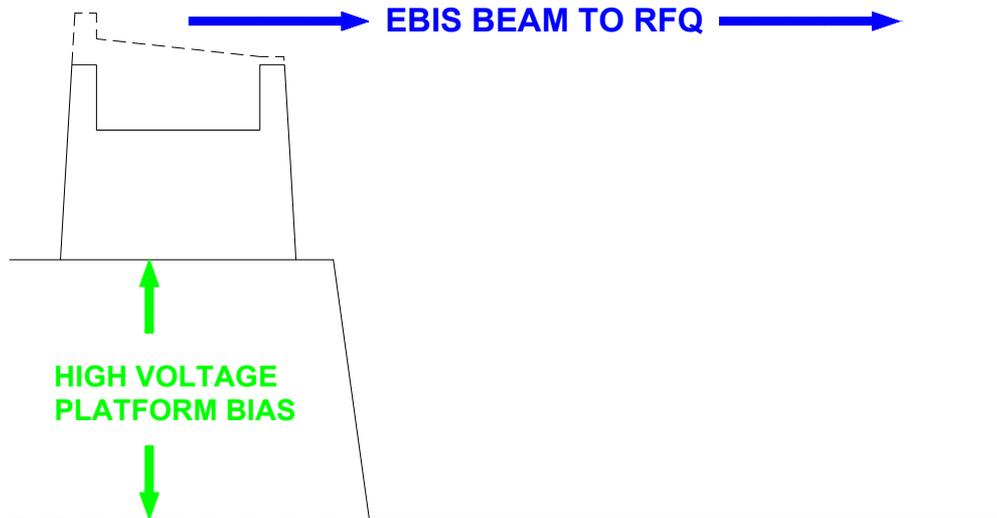
Just before ion extraction the EBIS Platform Voltage is applied such that the ions are extracted through 100kV (nominal) to attain the  $\sim 17\text{keV/amu}$  needed for acceleration by the RFQ
