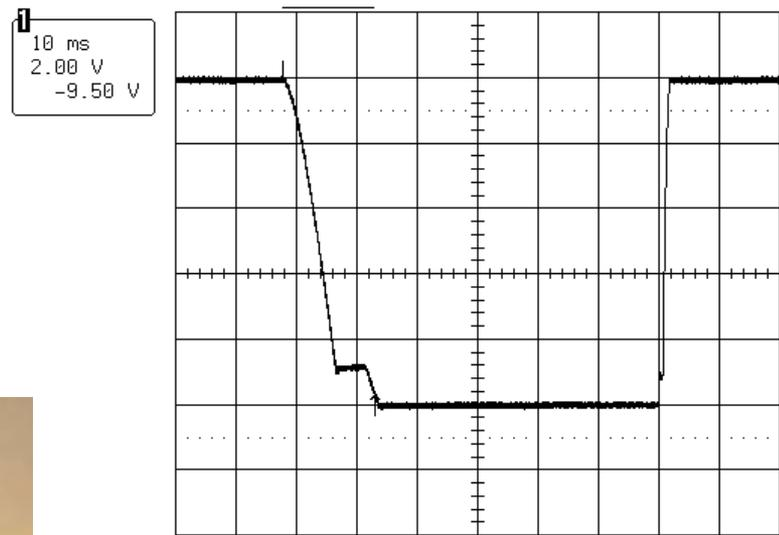
**10 A, 50 ms electron beam pulse**
