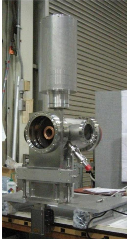
The new electron gun with the high perveance anode ( $\sim 3\mu\text{Perv}$ ) was installed and operated at the Test EBIS to produce electron beams up to 10A.
