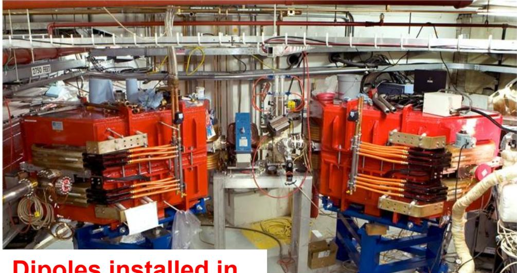
Dipoles installed in Booster (Sigmaphi)
