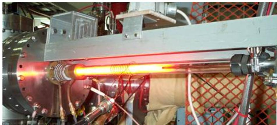
Hollow Cathode Ion Source (HCIS), based on design used on Saclay EBIS.
