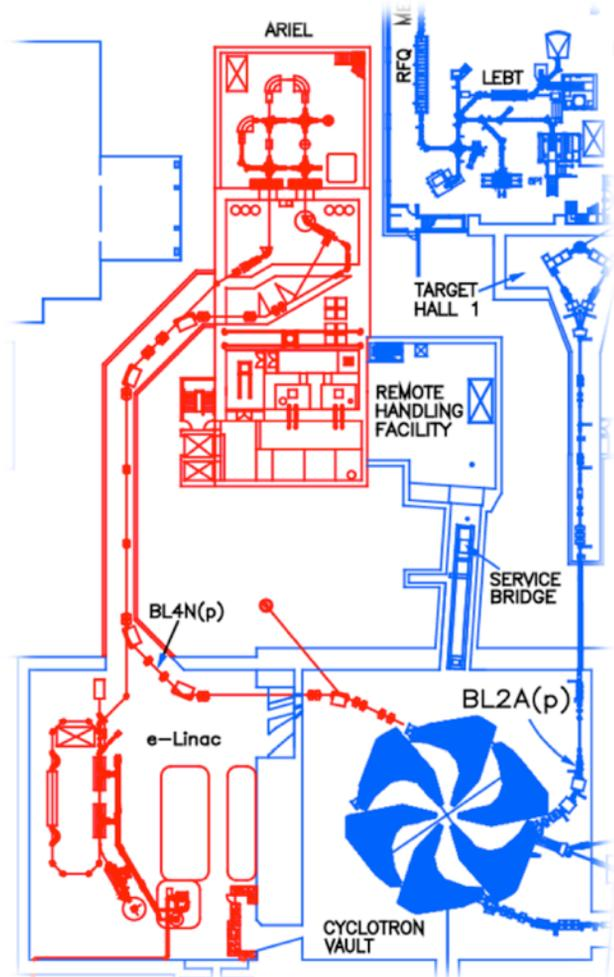
Figure 2: Beamline layout of the Advanced Rare Isotope Laboratory, showing its location relative to existing TRIUMF facilities. ISAC is at top right.
