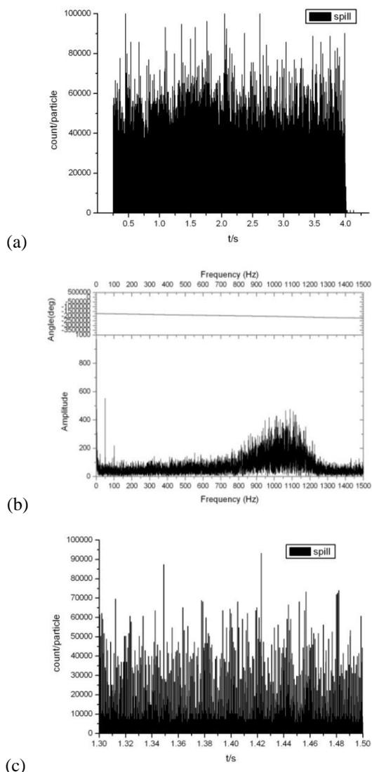
Figure 4: Spill in feedback mode(sample rate is 10 kHz). (a) Structure of one spill, (b)FFT of one spill, (c) Detailed spill structure in 1.3s-1.5s.
