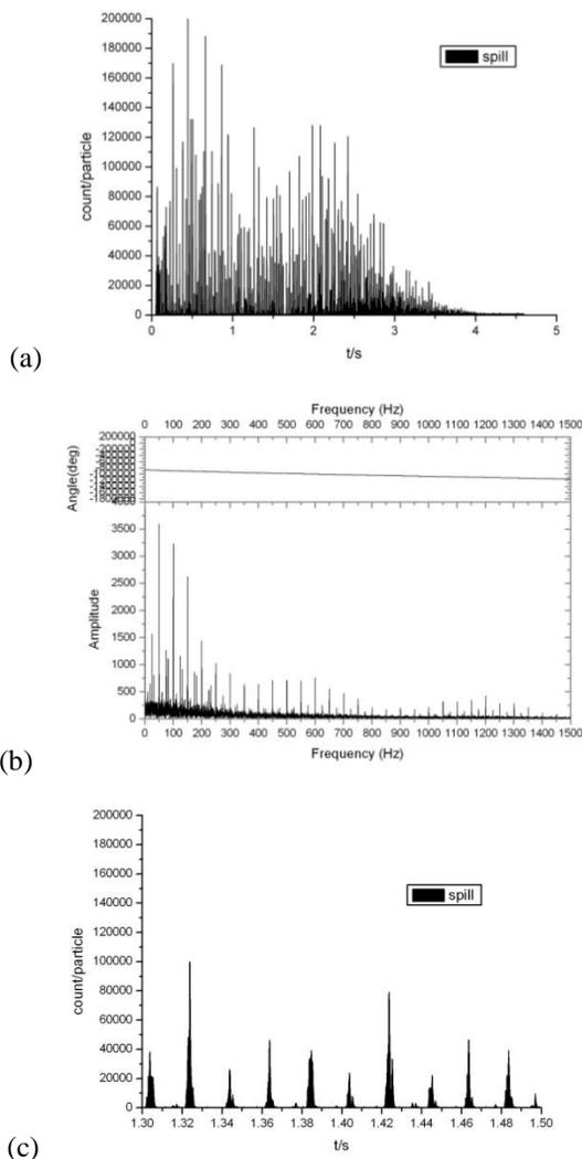
Figure 1: Spill in normal mode (sample rate is 10 kHz). (a) Structure of one spill, (b) The FFT of one spill, (c) Detailed spill structure in 1.3s-1.5s.
