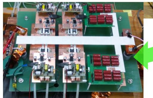
1.2/2.4 kV SiC-JFET Package developed by KEK/SunA
