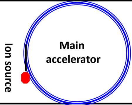
Functionally separated acceleration/confinement -> increasing a freedom of beam handling
