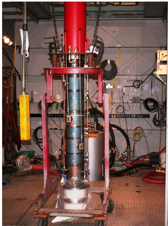
Figure 2: CPI VA-862A1 prototype klystron being installed in the test stand.
