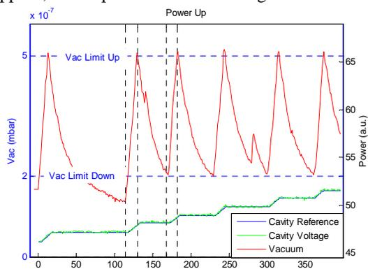
Figure 4: Automatic Conditioning of ALBA Dampy Cav.
