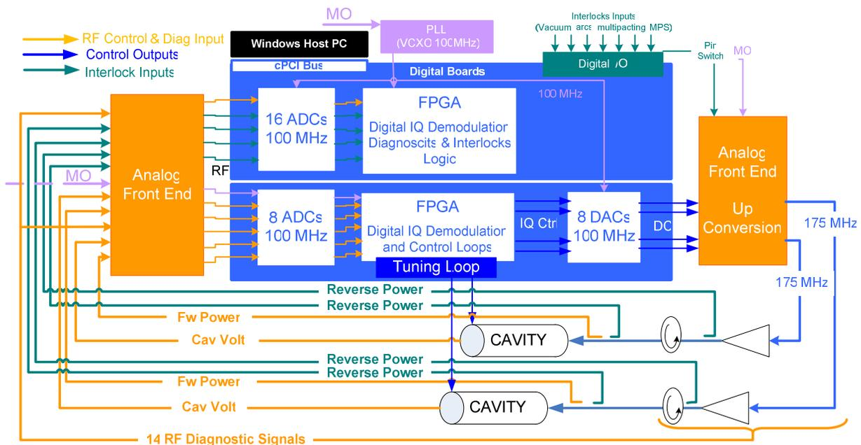
Figure 1: LLRF Hardware and Signals.
