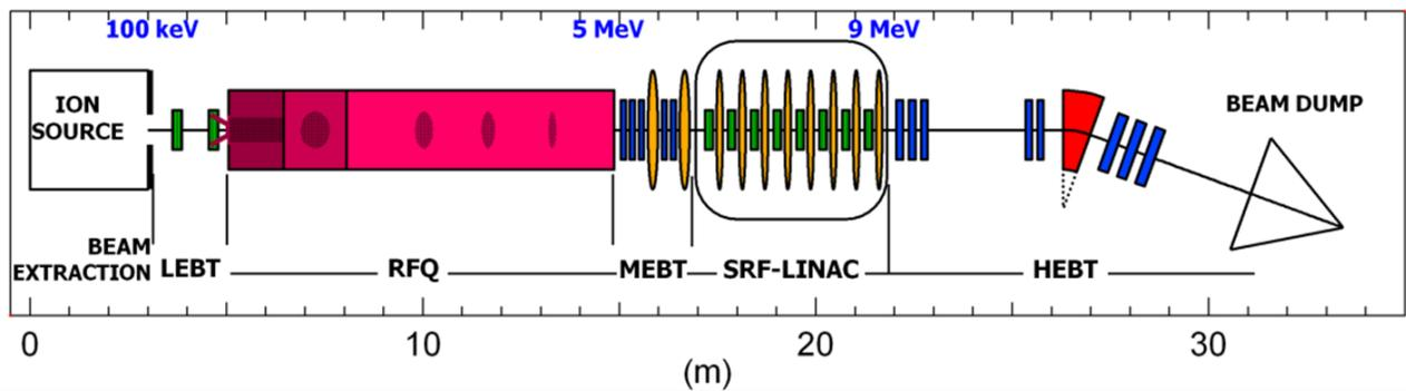
Figure 1: Scheme of the IFMIF-EVEDA prototype accelerator.
