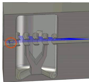
Figure 3: Final Focus cavity with shorting bars.
