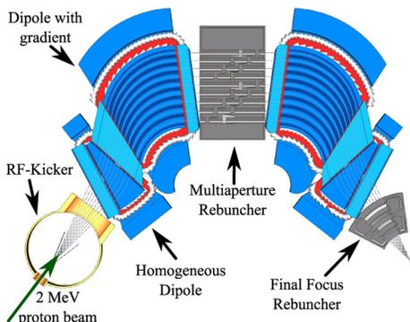
Figure 1: Design of the ARMADILLO. See [2] for details.
