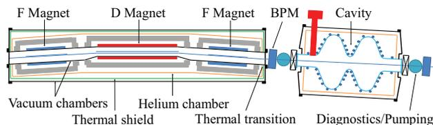
Figure 2: Layout of a single lattice cell containing an RF cavity.
