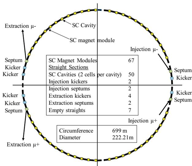
Figure 1: Layout of the FFAG ring.
