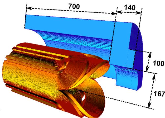
Figure 4: A design for the F magnet, showing half the magnet with dimensions in mm. Coils and an iron yoke are shown.
