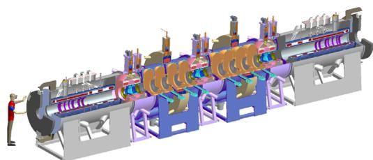
Figure 1: The MICE cooling channel and spectrometers.
