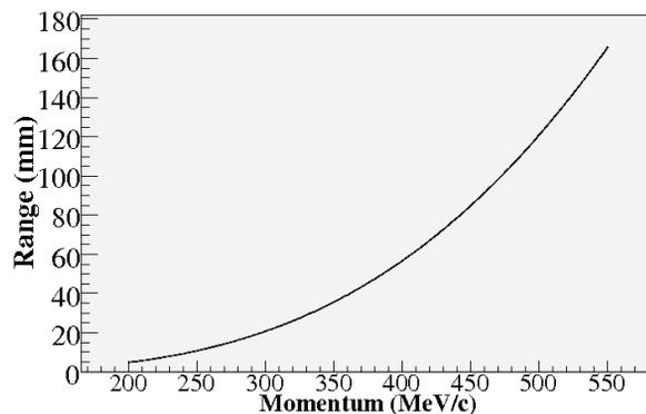
Figure 3: The range for protons in 0.89 g/cm<sup>3</sup> for momentum range of interest to MICE. This range was calculated by dividing the CSDA range, in g/cm<sup>2</sup>, obtained from [3] by the density of the MICE proton absorbers.
