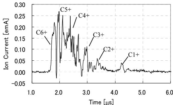
Figure 4: Single-shot TOF spectrum with potential barrier electrode. Laser energy 1.4 J, target to ion collector distance 2.5 m, and accelerating voltage 30 kV.
