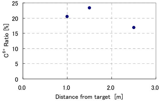
Figure 7: Dependence of C<sup>6+</sup> ratio on distance from target. Laser energy 1.4 J, and accelerating voltage 30 kV.
