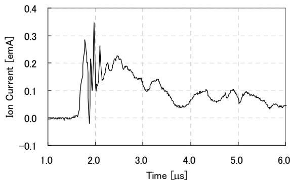
Figure 3: Single-shot TOF spectrum at without potential barrier electrode. Laser energy 1.4 J, target to ion collector distance 2.5 m, and accelerating voltage 30 kV.
