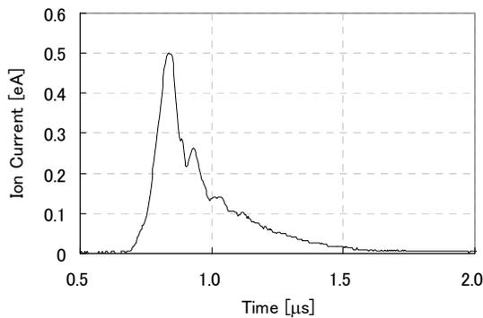
Figure 8: Single-shot current at acceleration electrode. Target to acceleration electrode distance was 10 mm, and accelerating voltage was 30 kV.
