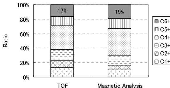
Figure 5: Ratio of each charge state. Laser energy 1.4 J, target to ion collector distance 2.5 m (target to MCP distance 2.2 m), and accelerating voltage 30 kV.
