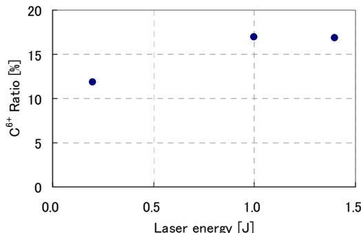
Figure 6: Dependence of  $C^{6+}$  ratio on laser energy. Target to ion collector distance 2.5 m, and accelerating voltage 30 kV.
