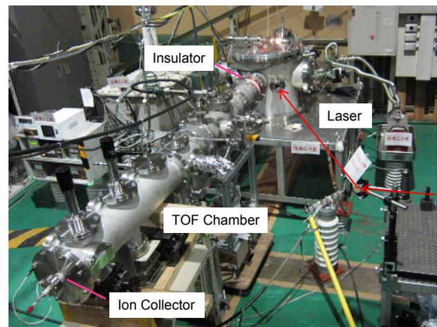
Figure 2: Photograph of the TOF setup.
