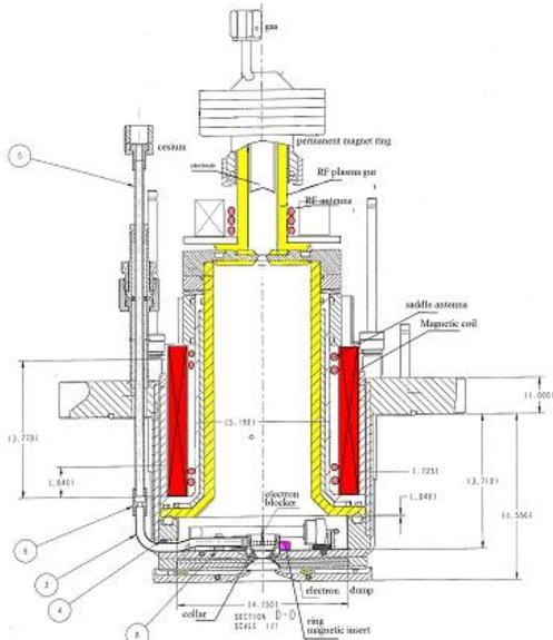
Figure 1: Upgraded design of the Advanced RF Saddle antenna SPS with RF plasma gun for pulsed RF discharge triggering (yellow-ceramic AlN; red-magnetic coil; orange-saddle antenna; magenta-magnetic insert ring).
