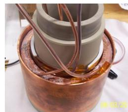
Figure 6: Water cooled saddle antenna and magnetic coil for high duty factor operation.
