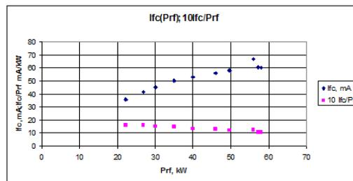
Figure 5: Evolution of the Faraday cup current  $I_{fc}$  and ratio  $I_{fc}/P_{rf}$  as function of  $P_{rf}$  during cesiation. The efficiency of  $I_{fc}$  generation increased with decreased gas flow Q from 20 sccm to 17.2 sccm.
