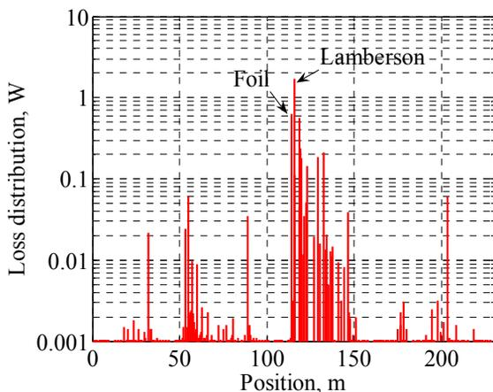
Figure 7: Beam loss distribution around the ring due to the foil scattering.
