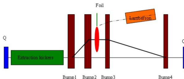
Figure 2: Layout of the foil scattering extraction system.
