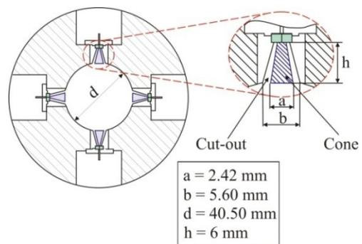
Figure 1: Cross-section of the cone-shaped pickup
