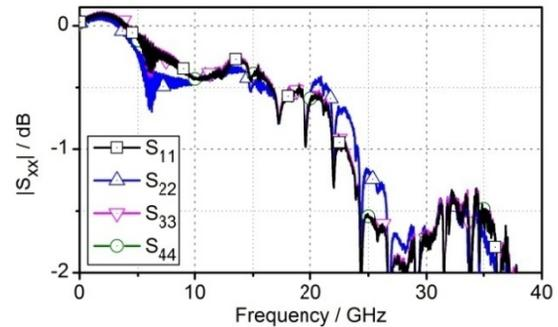
Figure 3: Reflection coefficients measured at the connectors.
