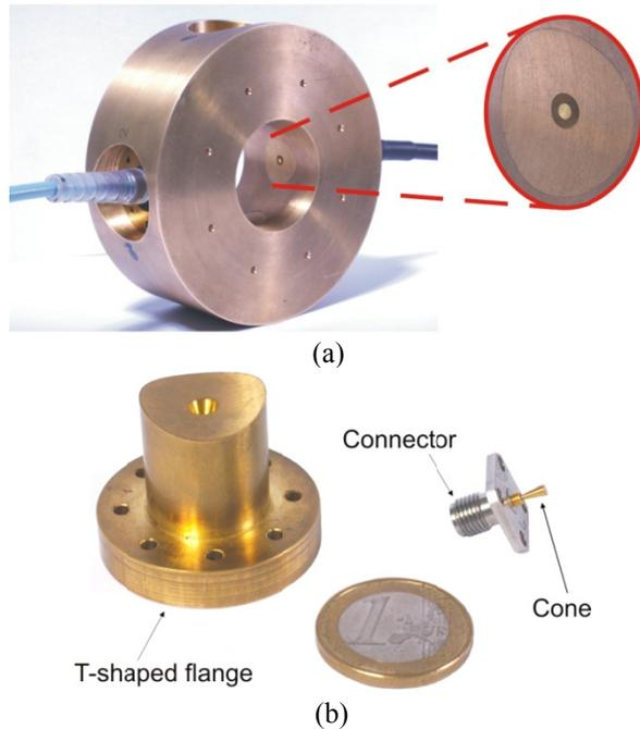
Figure 2: a): Photo of the non-hermetic cone-shaped pickup, b): T-shaped flange, the cone with the glass bead and the connector.
