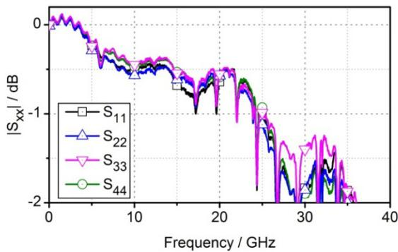
Figure 4: Reflection coefficients measured at the connectors with exchanged cones between port two and port three.
