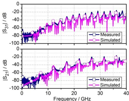
Figure 5: Cross-talking, measured vs. simulated.
