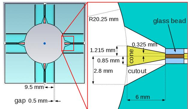
Figure 1: Reference dimensions of the cone-shaped design.
