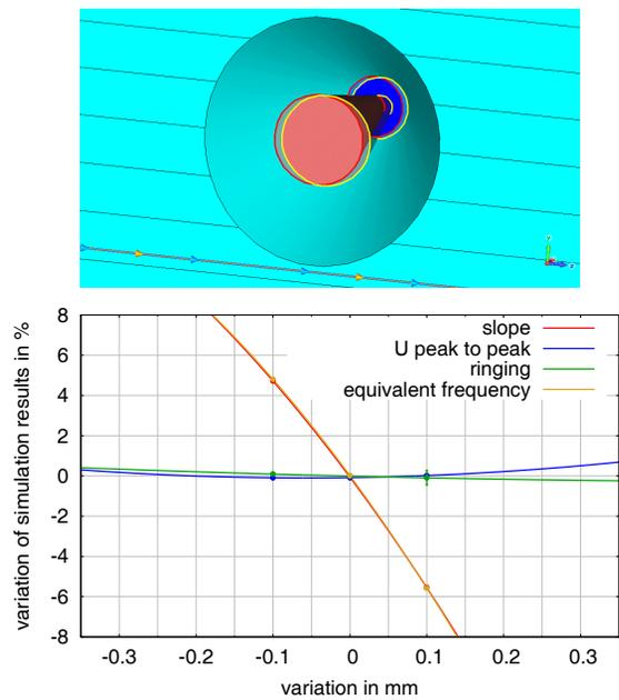
Figure 6: Variation of the position of the glass bead parallel to the beam axis and quadratic fit.
