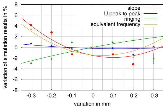
Figure 5: Tilting of the cone parallel to the beam axis and quadratic fit.
