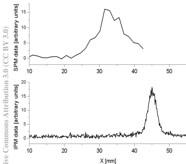
Figure 1: Comparison of the horizontal beam profiles acquired by the SPM (top plot) and the IPM (lower plot).
