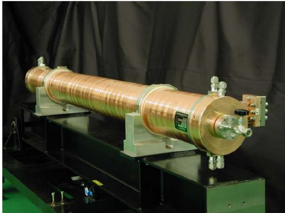
Figure 2 : C-band choke mode accelerating structure
