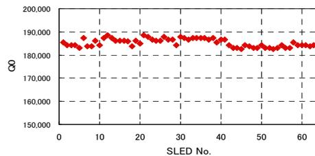
Figure 6 :  $Q_0$  measurement for all units.
