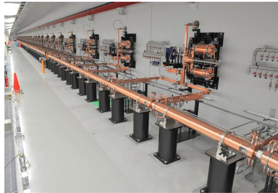
Figure 9: Installation of C-band section (by RIKEN).
