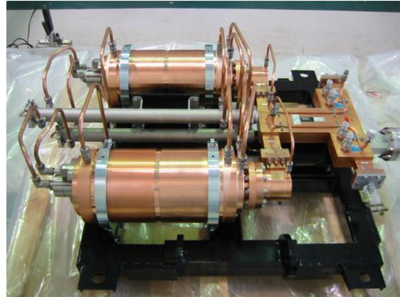
Figure 5 : C-band RF pulse compressor
