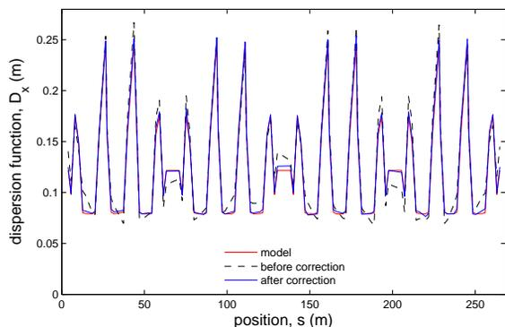
Figure 5: Horizontal dispersion function before (black) and after (blue) the LOCO symmetrization: the last iteration is very close to the model (red).
