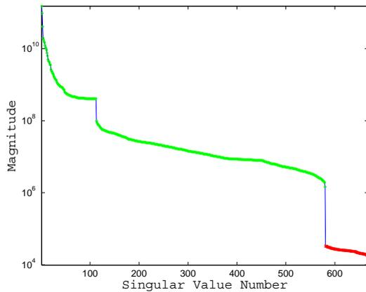
Figure 2: Spectrum of the singular values for the uncoupled LOCO fit with rejection threshold  $10^{-6}$ : retained values are shown in green, rejected in red.
