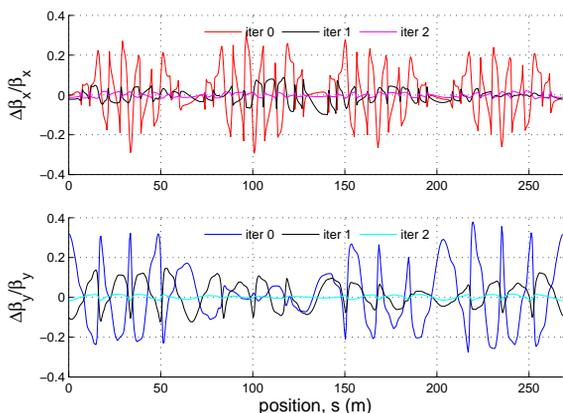
Figure 6: The horizontal (top) and vertical (bottom) beta beating in two symmetrizations of the optics is corrected from 30% (peak-to-peak) to 2% in both planes.
