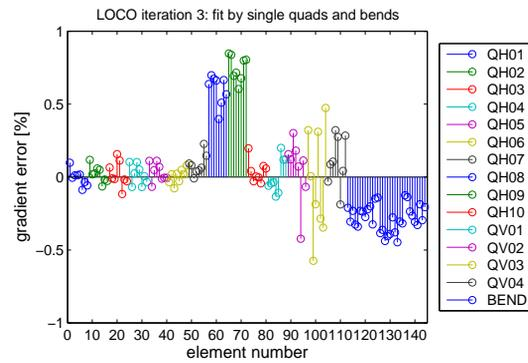
Figure 3: Calibration errors in the 112 quadrupole and 32 gradient dipoles fitted by LOCO.
