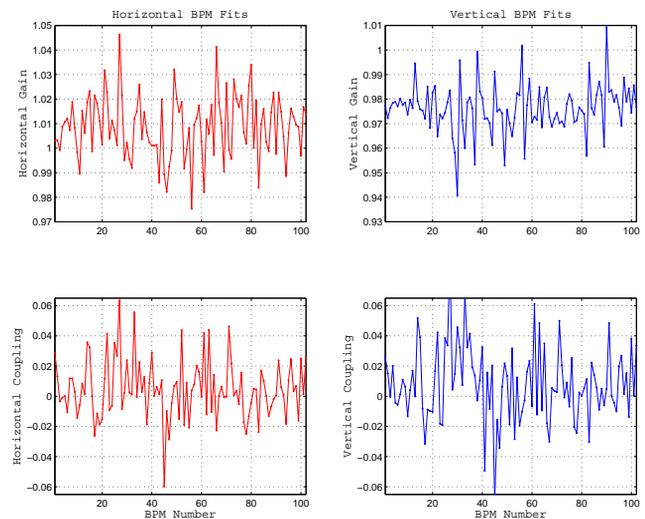
Figure 4: BPM gains (top) and coupling factors (bottom) in the horizontal (red) and vertical plane (blue).
