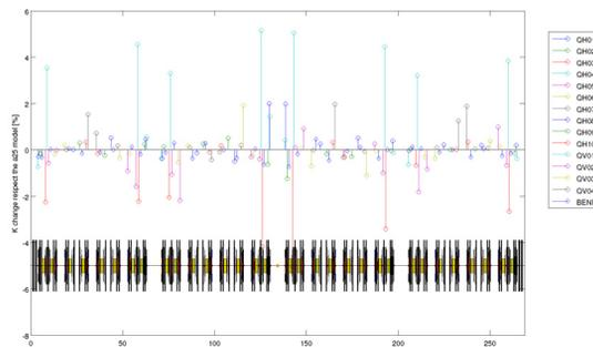
Figure 7: Total quadrupole gradient corrections applied to the storage ring to symmetrize the optics. Variations are within 1%, except the doublet of focusing quadrupoles QH03 and QH04 of the matching sections without BPM in between, where the changes are fighting each other and have drifted up to 4%.
