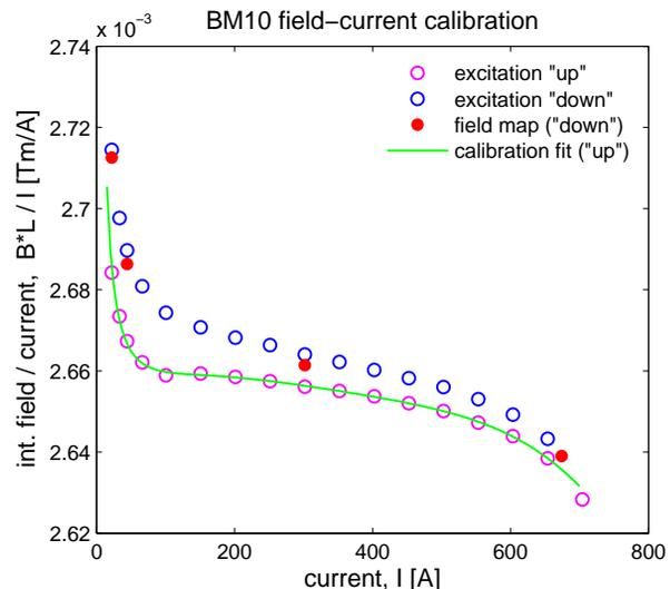
Figure 1: Long dipole BM10. Integrated field over current as a function of the excitation current.
