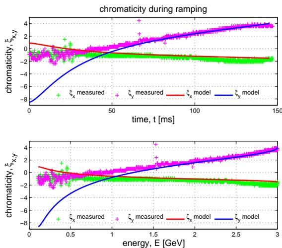
Figure 4: The measured and the theoretical horizontal and vertical chromaticity along the ramp as a function of the time (top) and of energy (bottom).
