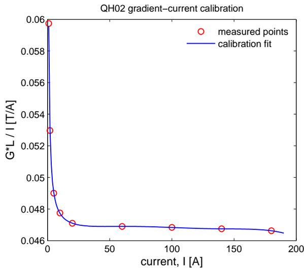
Figure 2: Integrated gradient over current factor for quadrupole QH02.
