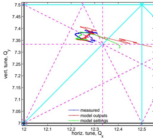
Figure 3: Movement of the working point during the ramp against the time (top) and plotted in the resonance diagram (bottom). The tunes measured from turn-by-turn data (blue line) are compared with the tune simulated with the model from the read-back currents (red line) and from the set currents (green line) of the digital power supplies.
