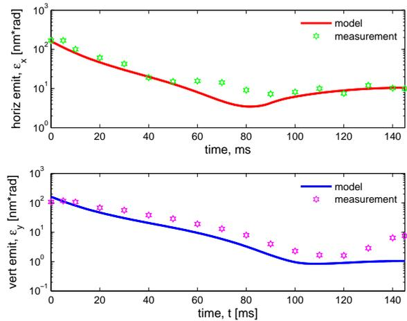
Figure 5: Horizontal (top) and vertical (bottom) emittance measurements during the ramp compared with the model.
