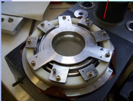
Mo electrodes, ~5 cm diameter, ~2000 holes, 0.8mm diam each, 3 gap (accel/accel/decel)
