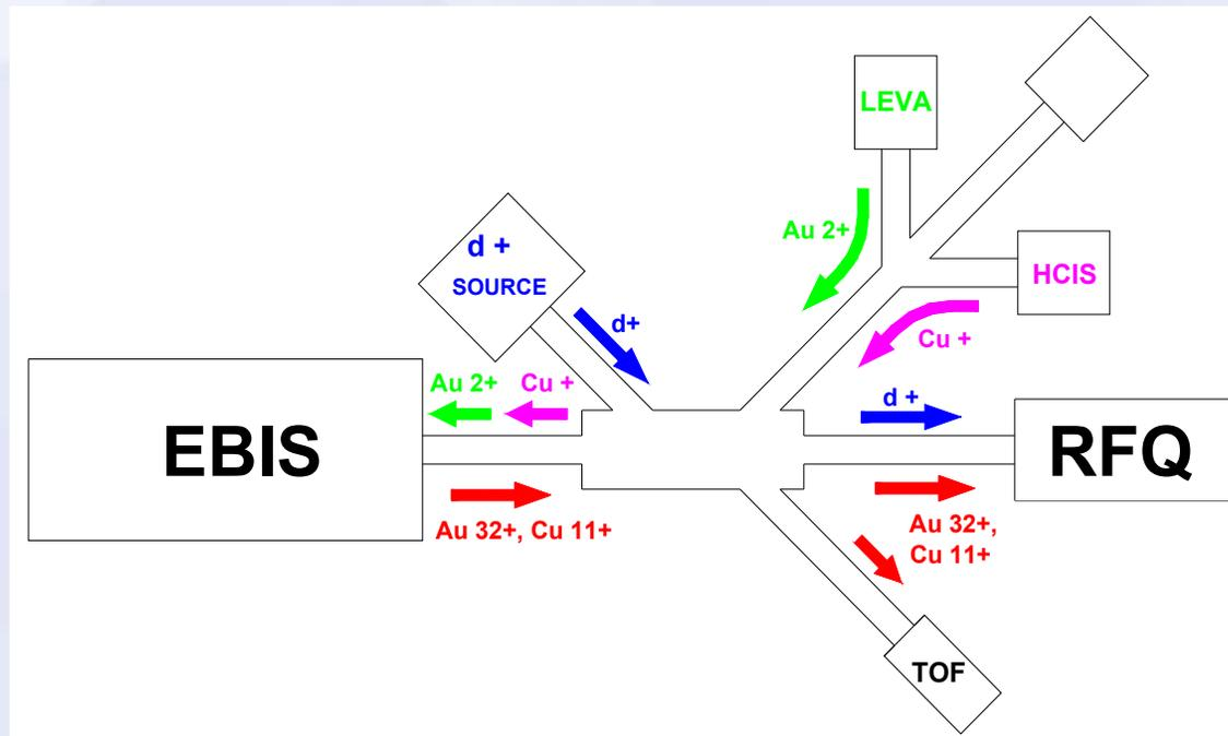
**External ion injection** provides most ion species (~ a charge breeder).
