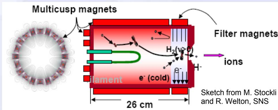
Filaments – ok for Cs-free sources, but output is low and electron current is high without Cs.
