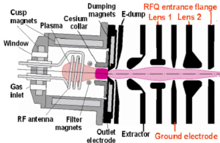
FIGURE 1. Schematic of the LBNL ion source and LEBT.
