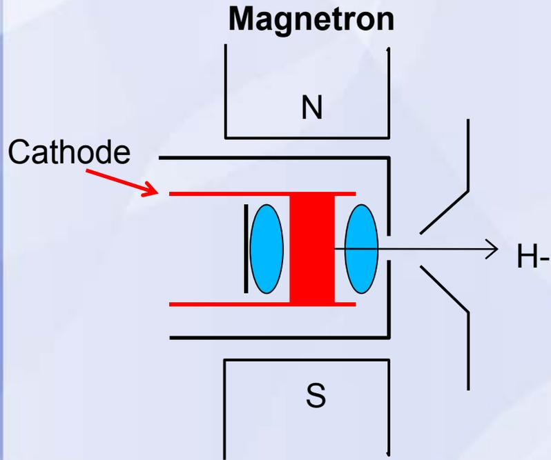
Plasma produced by ExB motion of electrons
