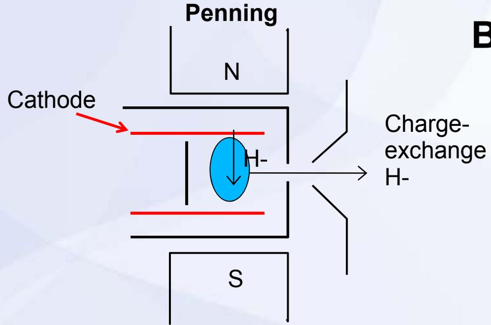
Plasma produced by electrons oscillating along the magnetic field, between two cathodes
