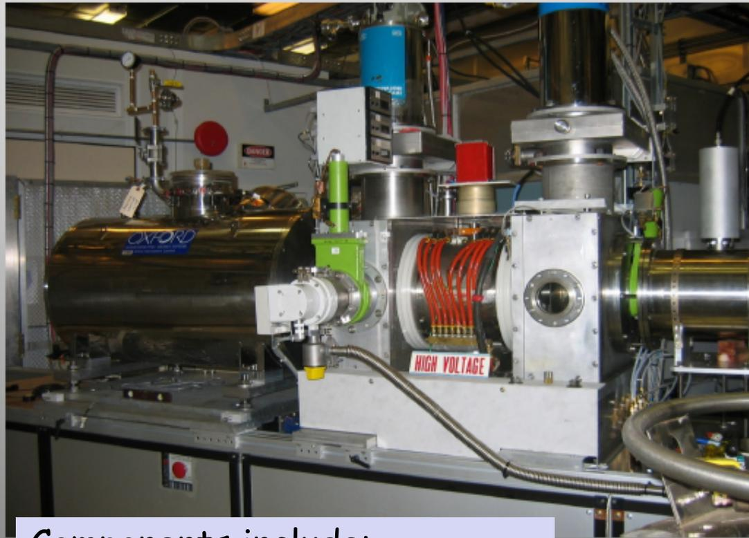
RHIC OPPIS produces reliably 0.5-1.0mA polarized H<sup>-</sup> ion current.
