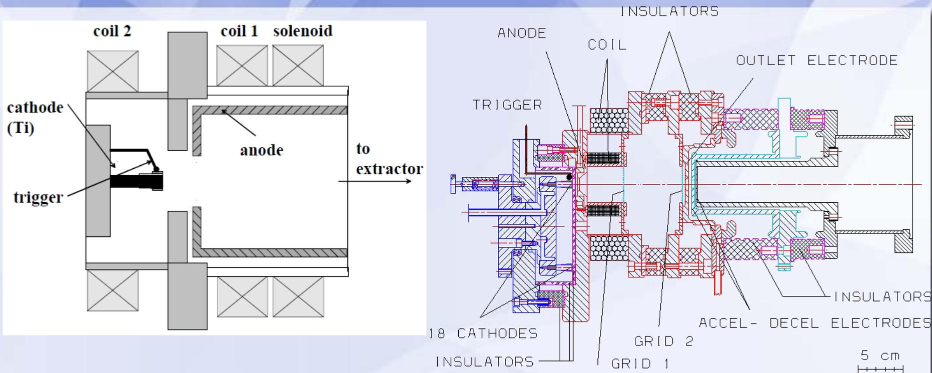
MEVVA having two additional coils, co-linear to the active cathode to influence the discharge impedance (increase the discharge current to the order of 1000A).
