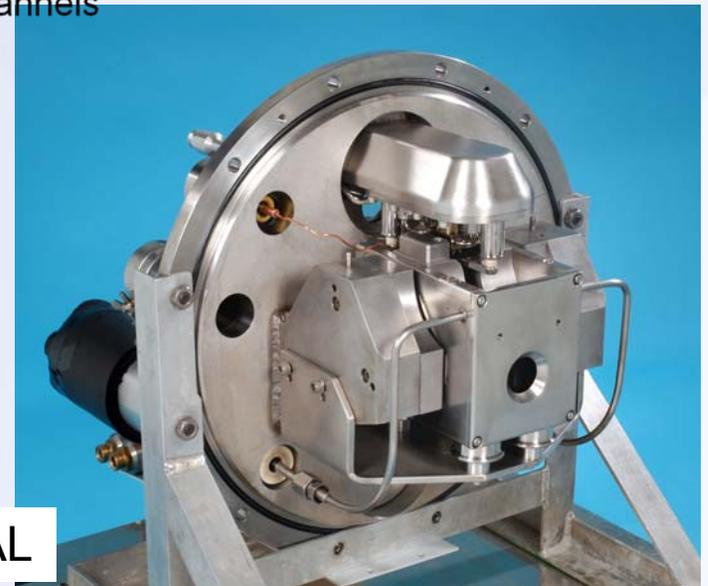
The ISIS operational ion source routinely produces 55 mA of  $H^-$  ions during a 200-250  $\mu s$  pulse at 50 Hz for uninterrupted periods of up to 50 days. The average lifetime of a source is about 21 days.
