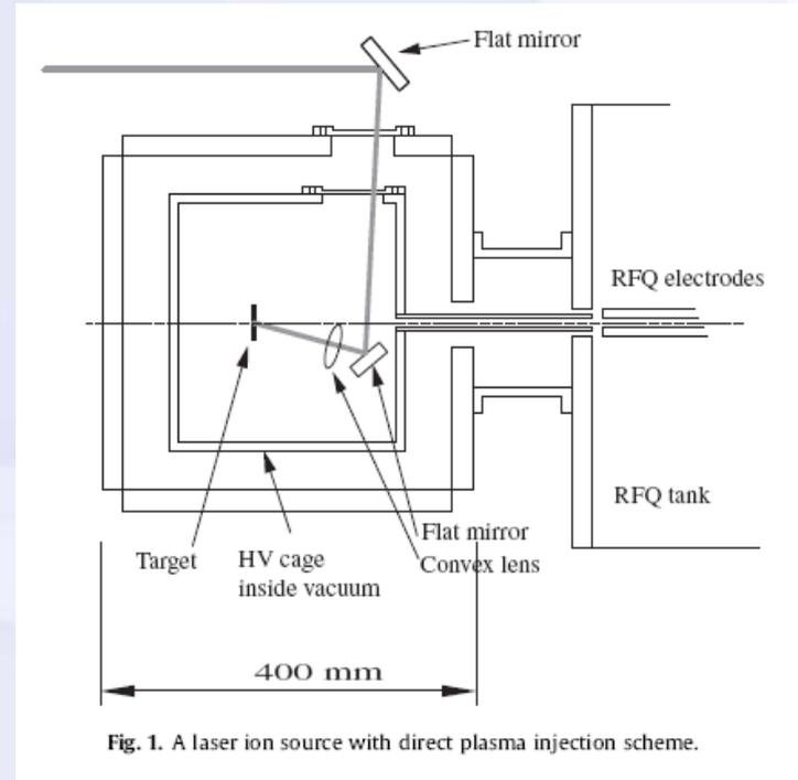
Fig. 1. A laser ion source with direct plasma injection scheme.
