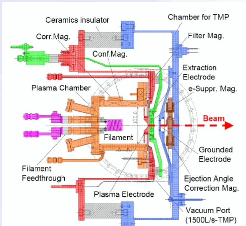
Figure 1: Cross-sectional view of the present J-PARC ion source.
