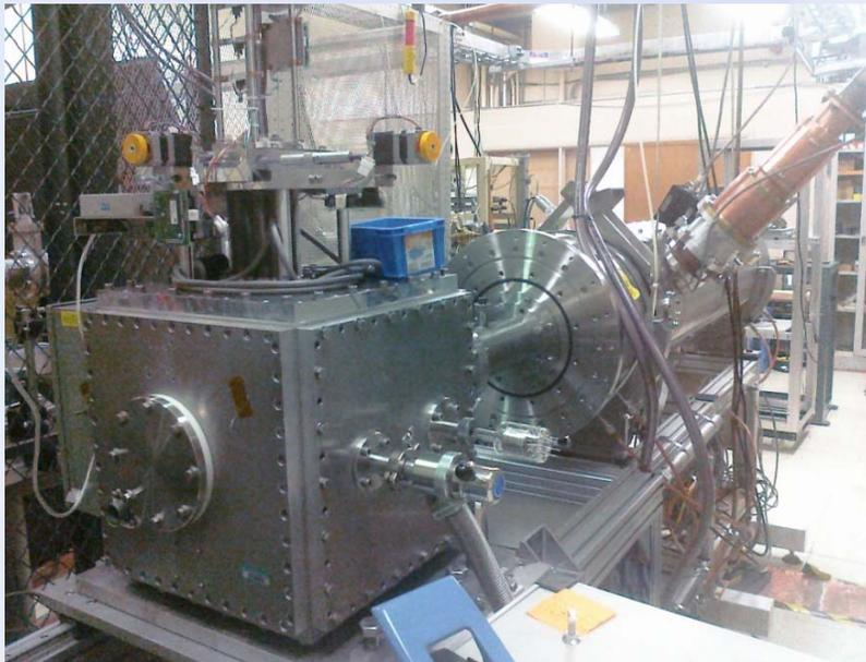
Allow a laser-produced plasma, containing the heavy ions of interest, to drift to the entrance of an RFQ, where the ions are then accelerated. This avoids the problem of space charge in matching a high current source to a subsequent accelerator. Ion extraction from the plasma occurs within the RFQ,
