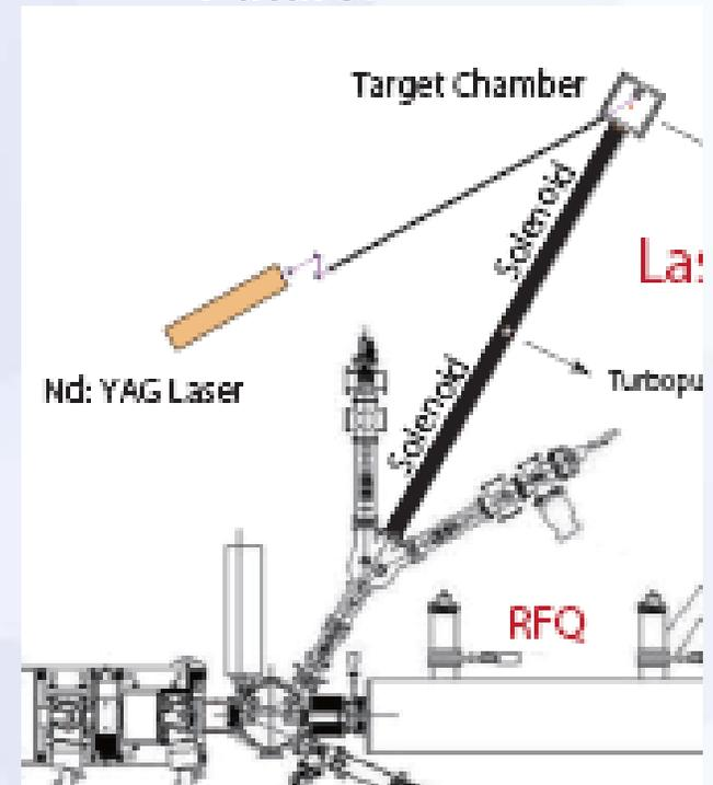
**LIS** - in a given pulse, laser irradiates any one in an array of target materials, to inject 1+ ions of that species into EBIS. This will allow fast switching of a larger number of species (R&D phase; supported by NASA)
