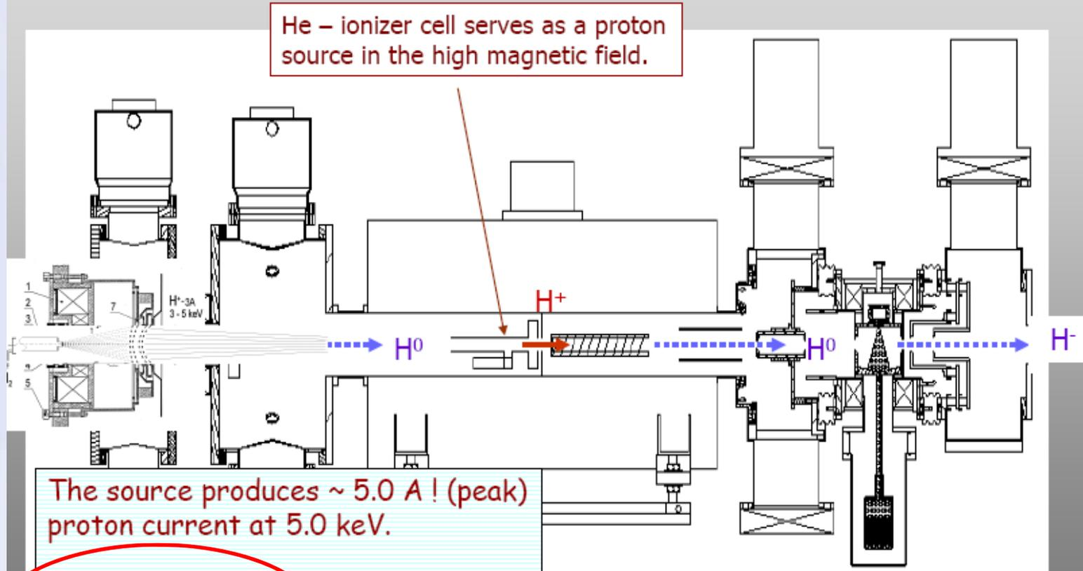
The source produces ~ 5.0 A ! (peak) proton current at 5.0 keV.
