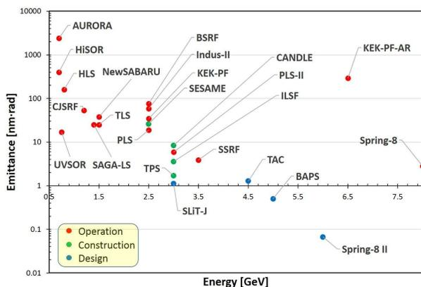
Figure 2: Synchrotron light sources in Asia, emittance V.S. energy.
