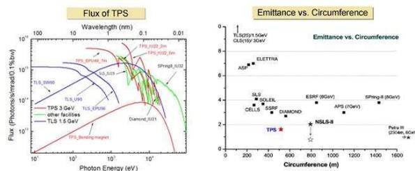
Figure 5: TPS will be the next new light source, with ultra low emittance at 1.6 nm-rad@3 GeV.
