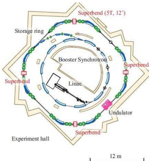
Figure 3: A 1.2GeV low energy compact light source CJSRF [12] is completed in Nagoya.
