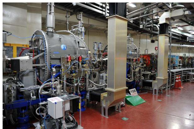
Figure 4: PLS-II upgrade project was completed in 2012, shown here is the newly installed superconducting RF sections.
