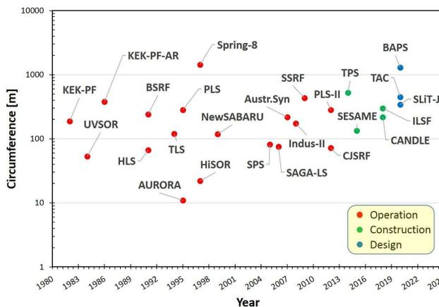
Figure 1: Synchrotron light sources in Asia, circumference V.S. completion year.
