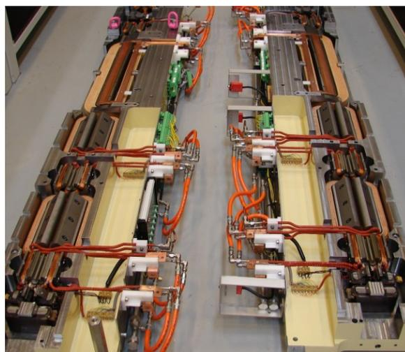
Figure 2: Top and bottom parts of an M1 magnet girder.
