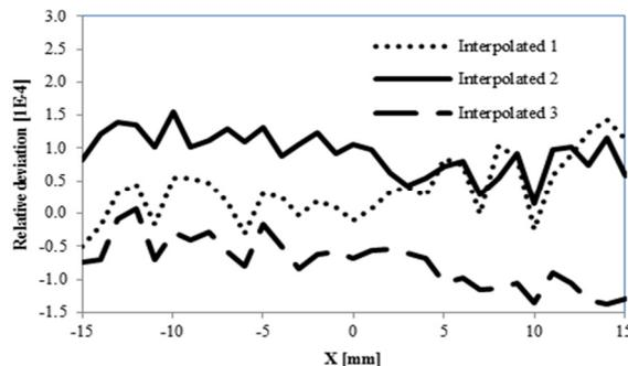
Figure 6: Relative deviation between discrete step-and-go measurements and interpolated field values on a transverse line of a combined function bending magnet.
