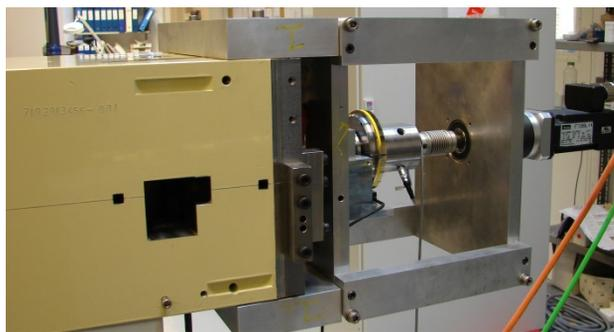
Figure 7: Rotating harmonic coil measuring system mounted on an end section with inserted pick-up coil.
