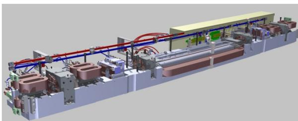
Figure 1: Mechanical layout for the U3 magnet girder.
