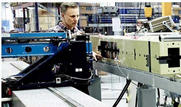
Figure 3: Field mapping with a Hall probe mapper on a granite bench with longitudinal axis along the beam axis.
