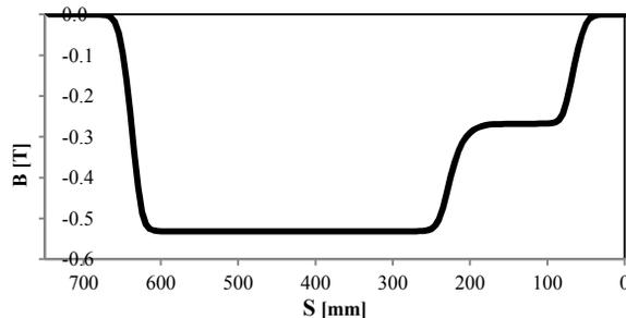
Figure 5: Magnetic field on the main orbit trajectory obtained by interpolation from the measured grid data.
