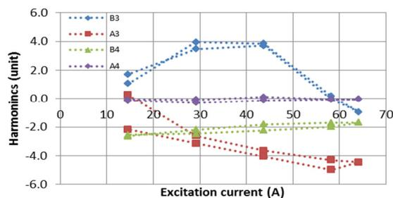
Figure 8: Measured normal and skew sextupoles (B3, A3) and octupoles (B4, A4) harmonics as a function of current for a focusing quadrupole on the M2 girder.
