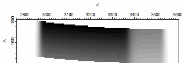
Figure 4: Magnetic field map of an M2 dipole. Darker color indicates higher field level.
