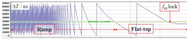
Figure 1: Time interval,  $\Delta T$ , between leading RF bucket of the two beams (scale is revolution time) during the ramp and cogging process at flat-top. The RF frequencies are locked together when  $\Delta T$  is close to the value placing the encounter points of the leading buckets at IP1, then a final adjustment is made (Figure 2).
