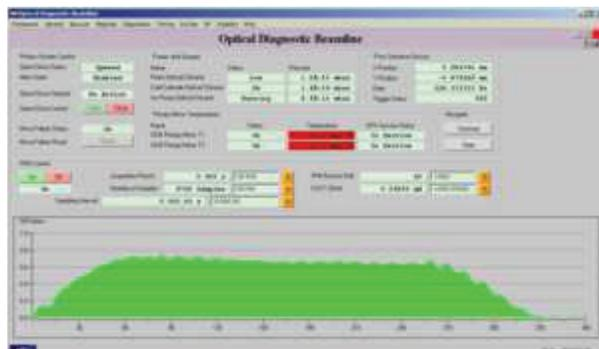
Figure 2: Typical user mode fill pattern.
