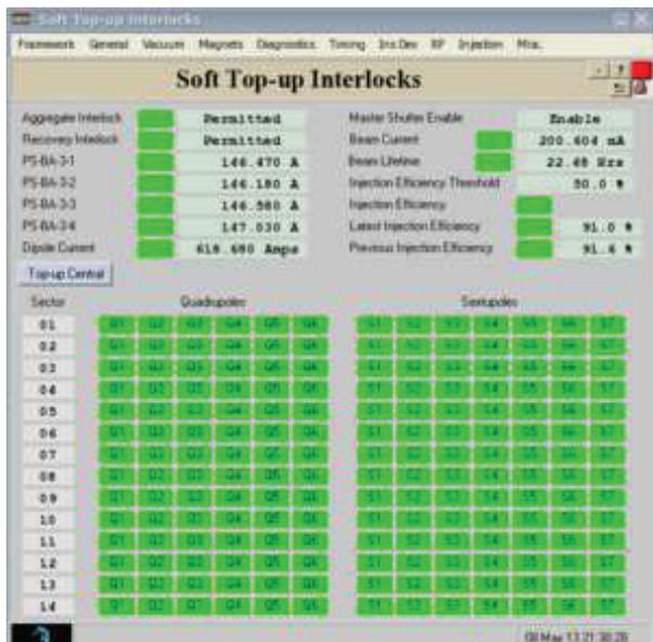
Figure 1: GUI for the top-up interlock and magnet monitoring system.
